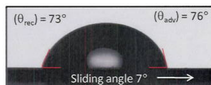
Figure 2. Sliding angle of a 10 \mu L drop of hexadecane rolling of Si wafer coated with compound 3 .
