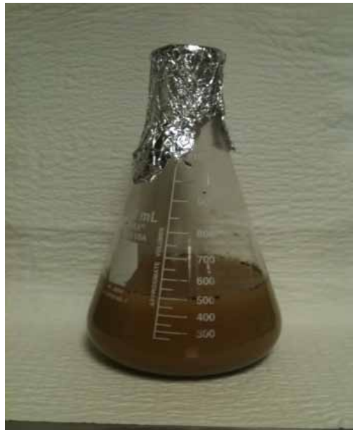
Figure 2. Mock up of bioreactor used in this study, an Erlenmeyer flask filled with soil and groundwater, spiked with contaminants and amendments.
