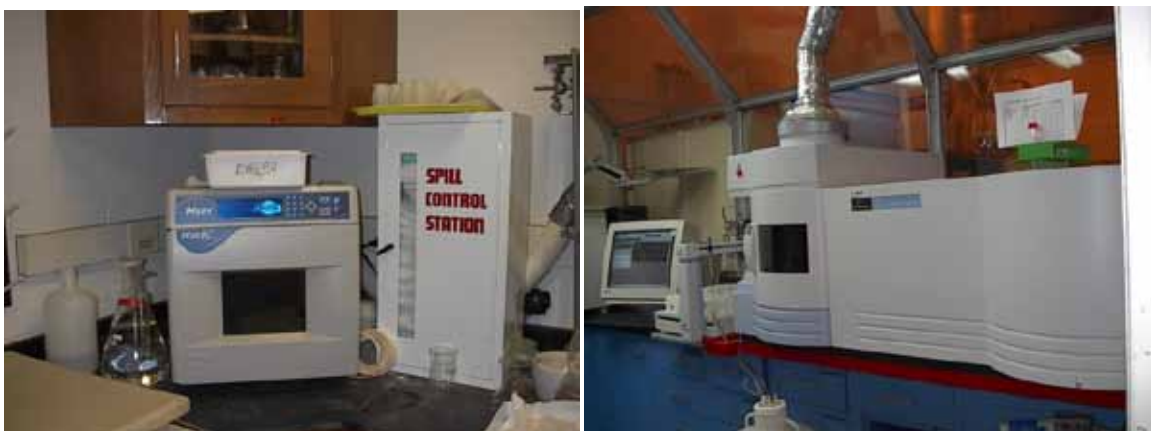
Figure 8. Microwave digester and ICPOES for analysis of metals.
