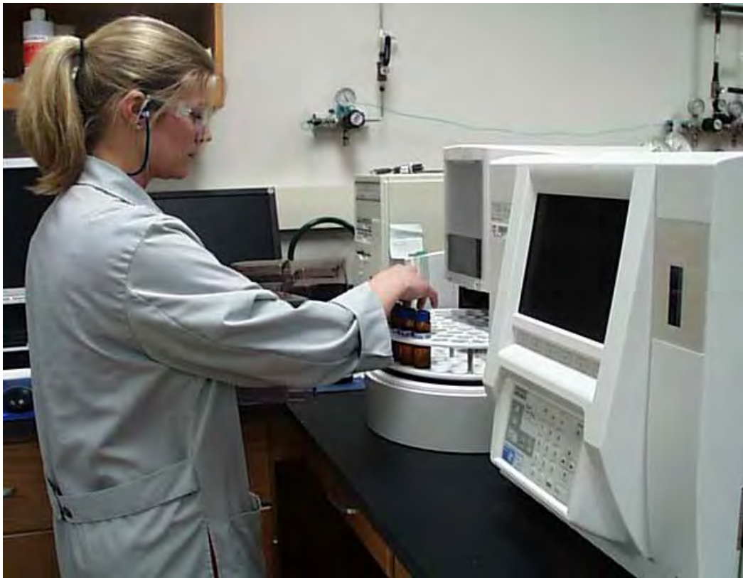
Figure 6. TOC instrument used during project. It is useful for quantifying organic material in sand/soil and for analyzing additives in groundwater.
