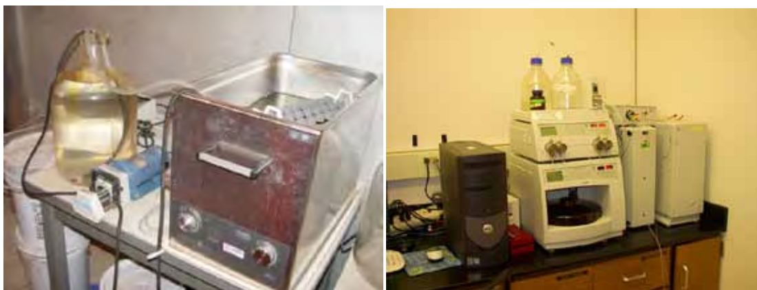
Figure 5. Temperature controlled sonicator used for extraction of explosives from aquifer sand/soil & a high pressure liquid chromatograph for explosives analysis.
