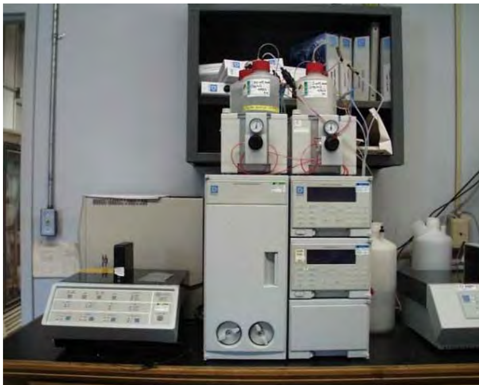
Figure 7. Ion chromatograph available for nutrient analysis.
