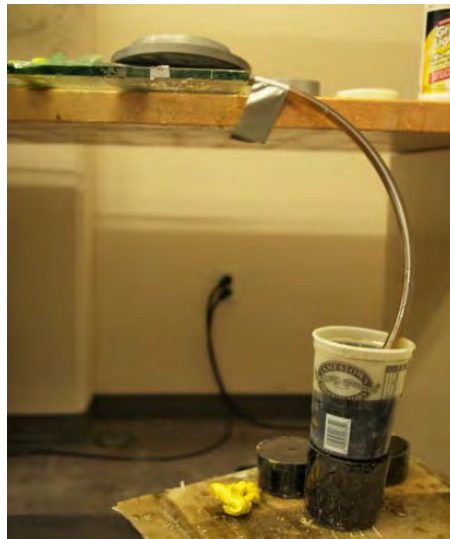
Figure 21. Polyethylene tube submerged in the resin reservoir with sealant tape removed.
