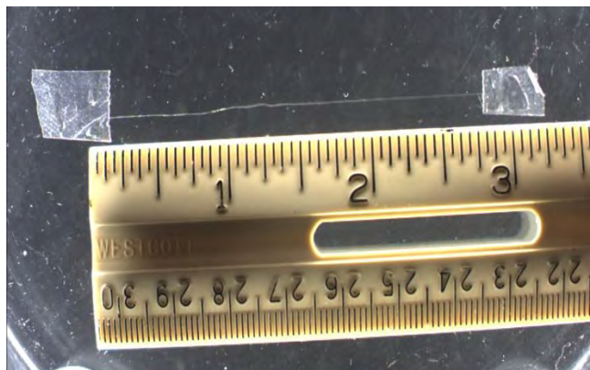
Figure 8. FLH fiber spun from a ~300 mg/ml solution in PT-0.2M arginine aged 2 days at 4°C. Fibers were sufficiently durable to handle after collection and prepared for optical and scanning electron microscopy.
