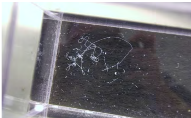
Figure 7. Aqueous spinning of FLH PT-100 mM glycine sample (500 mg/ml) in 50% methanol. Long, continuous fibers were formed and the fibers could be pulled within the bath.
