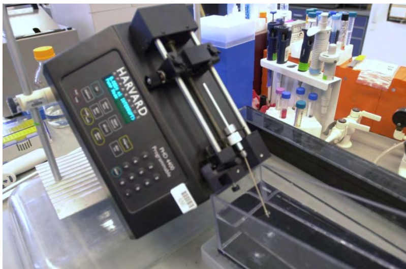
Figure 6. Aqueous spinning system is displayed with a coagulation bath and Harvard pump. Typically, a spin trial uses 50 \mu l of sample. After fiber formation, fibers are removed by hand with tweezers, if possible.
