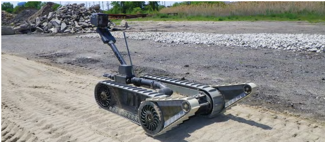
A small UGV undergoes battery testing on a test course in Clinton Township, MI. Advancing these systems' batteries will allow for greater power and enhanced technology to be integrated onto platforms. (U.S. Army TARDEC photo.)
