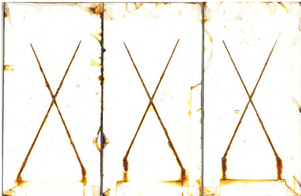
Figure 22. Control Coating SO 2 Corrosion Resistance Test Outcome – Steel
