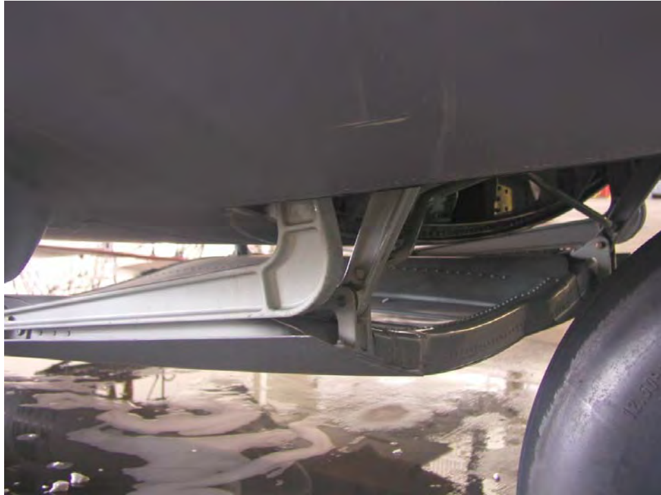
Figure 51. C-130 Nose Landing Gear Aft Door (AC: 92-1534) After 12 Months of Exposure
