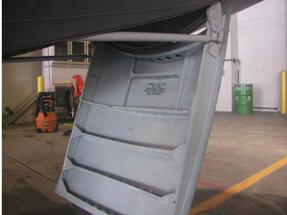
Figure 50. C-130 Nose Landing Gear Forward Door (AC: 92-1534) After 12 Months of Exposure
