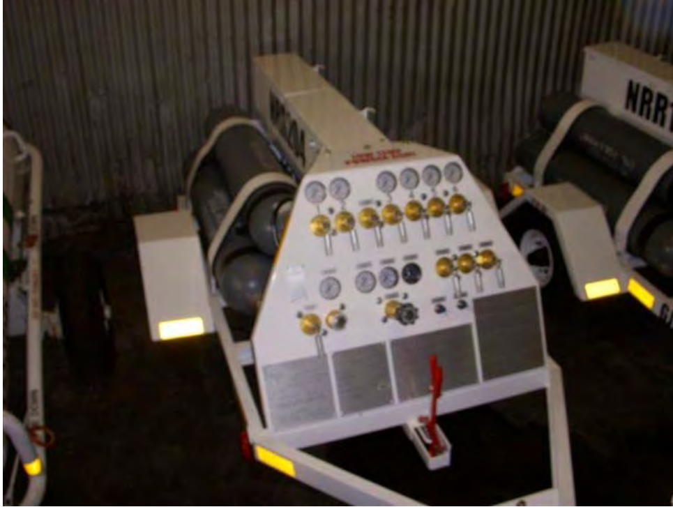
Figure 44. Nitrogen Servicing Cart (SN: NRR204) Prior to Carrier Exposure
