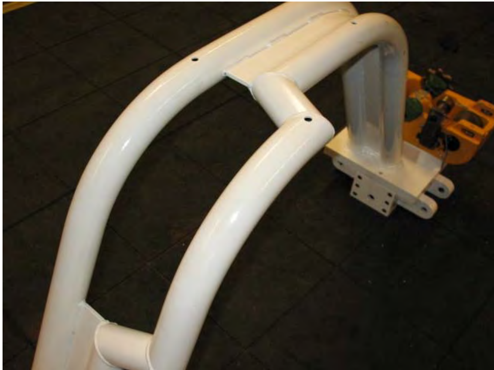
Figure 47. J52 Aft Engine Yoke (SN: P9H513) Prior to Coastal Exposure
