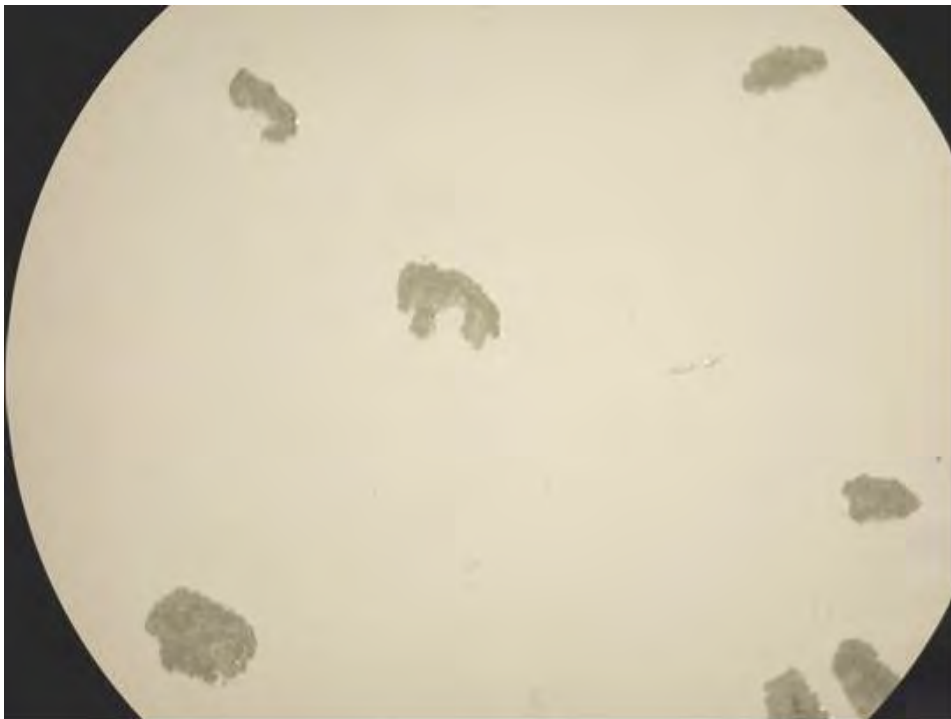
Figure 57. Control Coating Chipping Resistance Test Outcome
