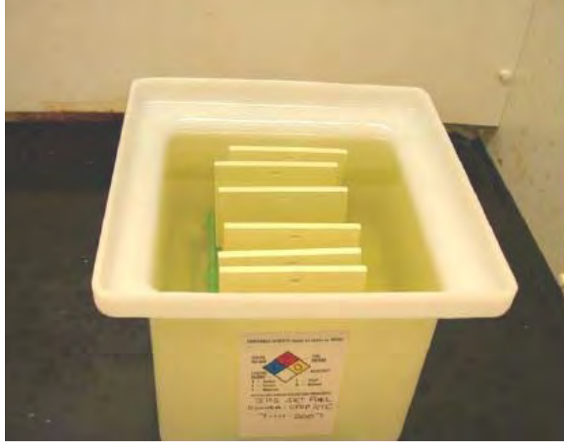
Figure 55. JP-5 Fuel Immersion Tank
