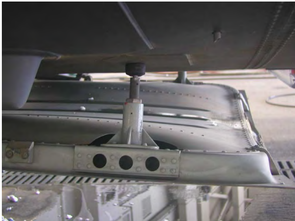
Figure 52. C-130 Nose Landing Gear Aft Door (AC: 92-1534) After 12 Months of Exposure
