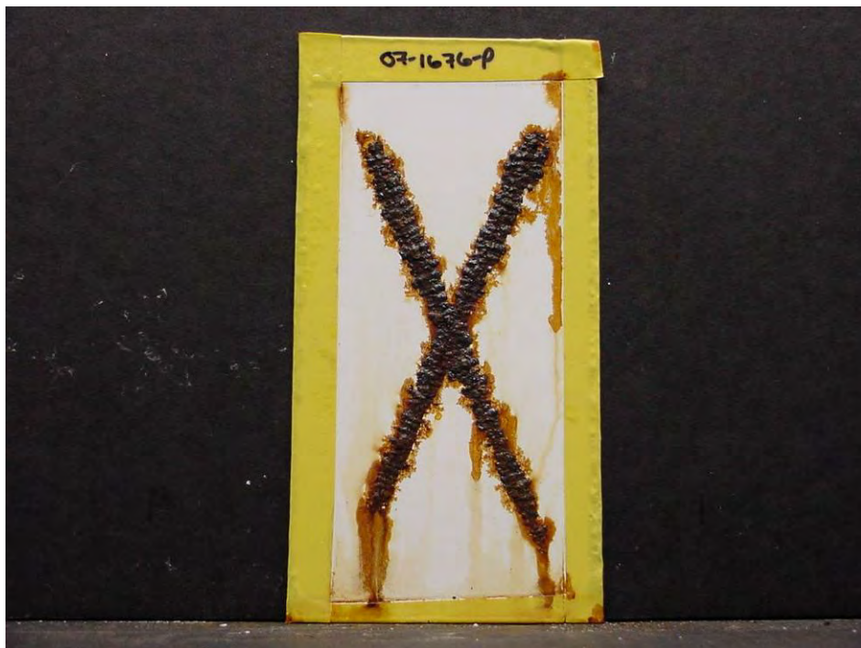
Figure 26. Control Coating Cyclic Corrosion Resistance Test Outcome – Steel
