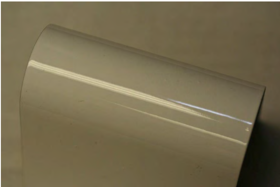
Figure 40. Control Coating Low Temperature Flexibility Outcome
