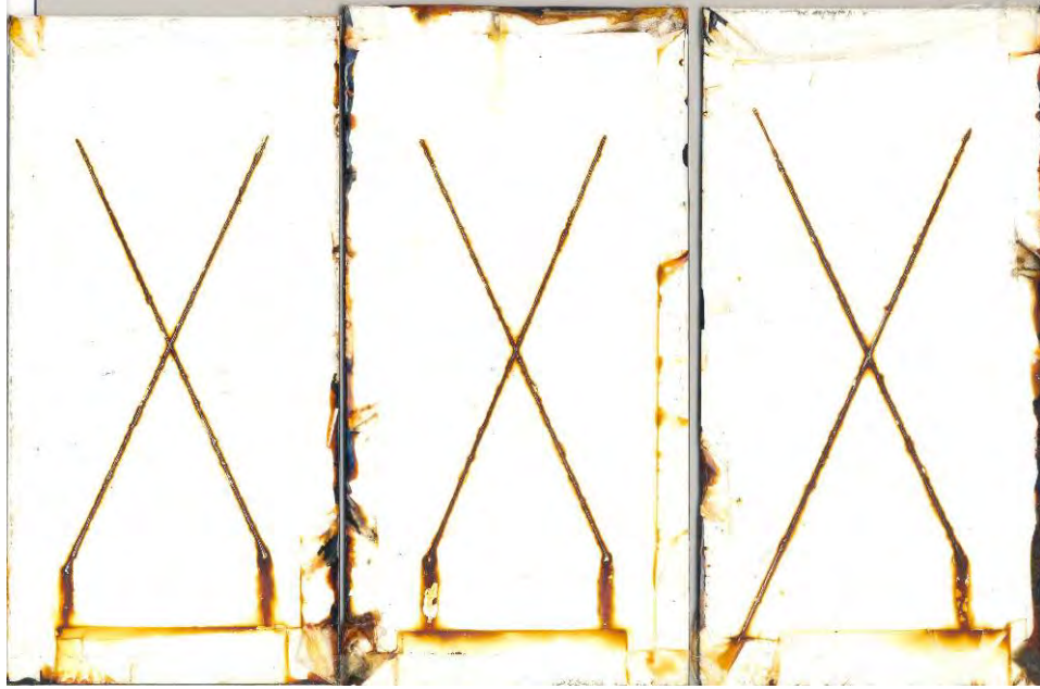
Figure 21. LTCPC SO 2 Corrosion Resistance Test Outcome – Steel
