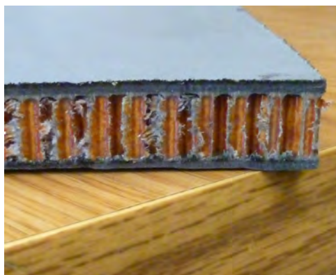
Figure 2b. Photo showing the cross section of an airframe sample used as the substrate in this project. The honeycomb structure is sandwiched in between two layers of metallic-polymer skins in light blue color.
