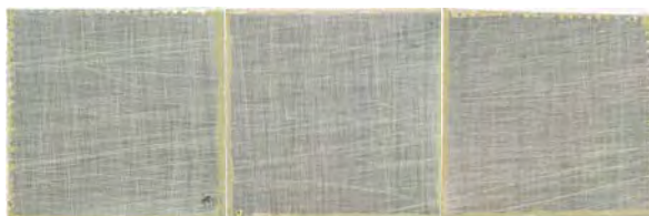
Figure 61. Aluminum panels after 30 minutes in methylene chloride with benzyl alcohol, ethanol, anhydrous acetic acid, and water.
