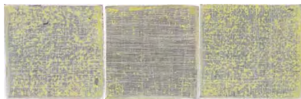
Figure 62. Aluminum panels after 30 minutes in methylene chloride with cyclohexanol, ethanol, anhydrous acetic acid, and water.
