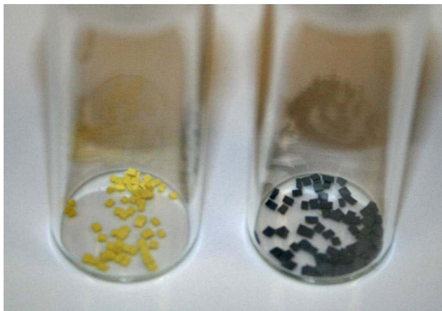
Figure 2. Examples of free-standing samples prepared for volume swell analysis; epoxy primer on the left, polyurethane topcoat on the right.
