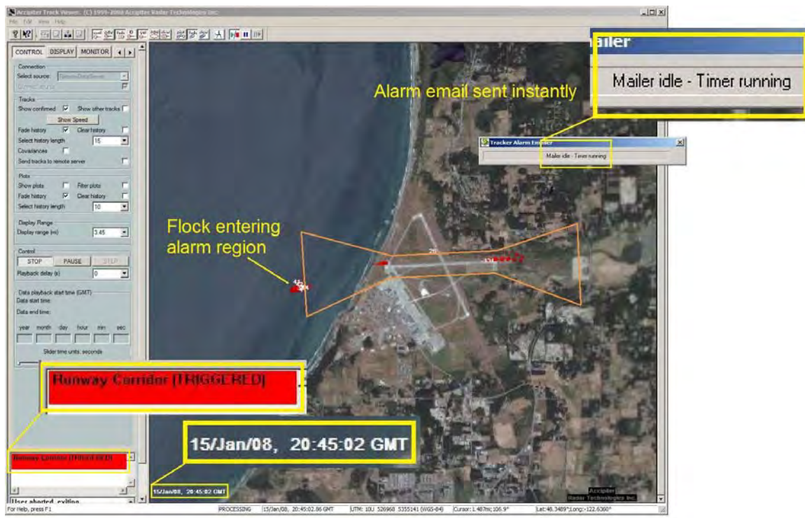
Figure 6-92. Alarm triggered as a flock of black-bellied plovers enters the alarm region set for NASWI on 25 January 2008.
