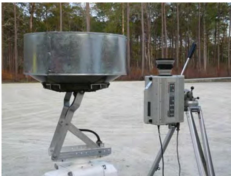
Figure B-10. The TI-VPR sensors: A Furuno FR2155-BB 50 kW X-band radar with a vertically-pointing parabolic dish (left), and Radiance I high-resolution thermal imaging camera (right).
