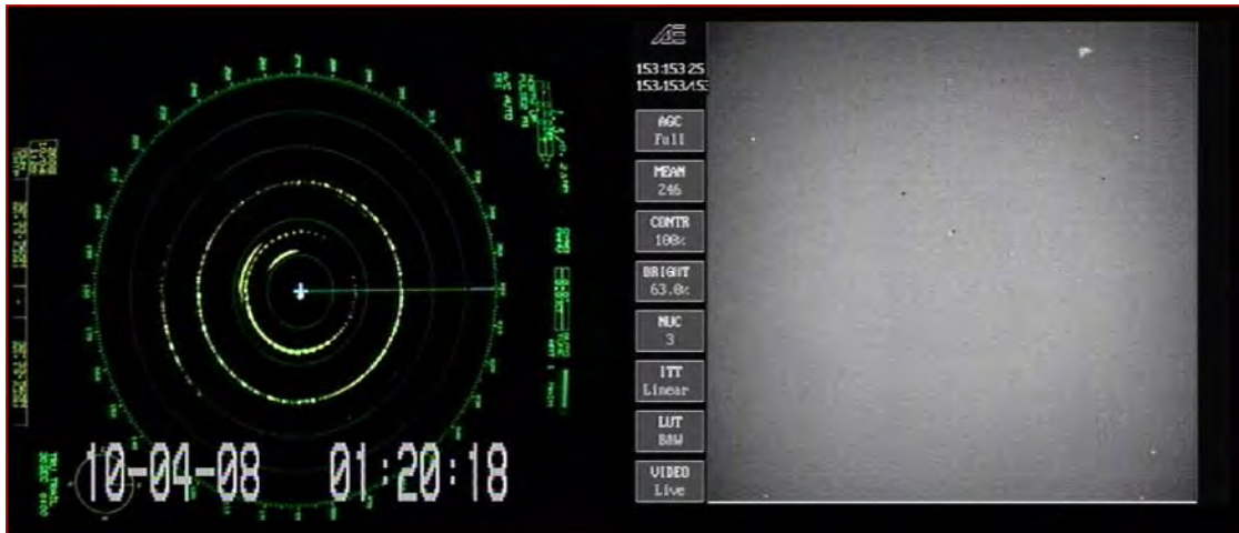
Figure B-12. Duplexed image showing radar image with date and time stamp (left) and thermal imaging camera display (right). Because the two images are video-duplexed, time synchronization is not a problem.
