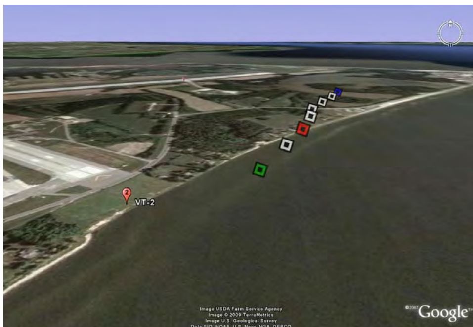
Figure 6-21. Trajectory of Track ID 111 at NAS Patuxent River, Maryland relative to site VT-2 that visually confirmed the target on 24 September 2008. The blue, red, and green placemarks denote the start, confirmed, and end positions of the target track, respectively.
