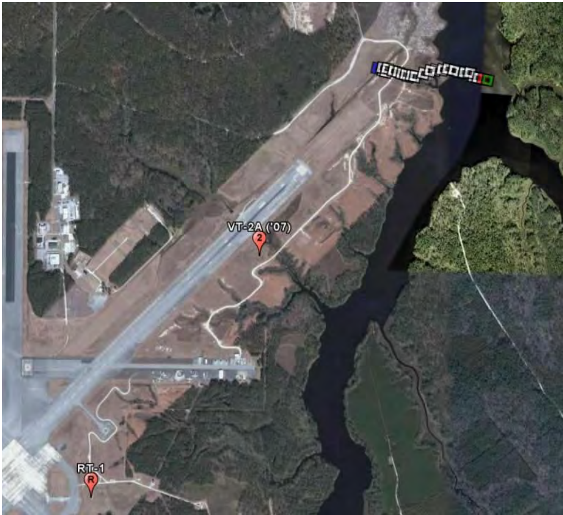
Figure 6-27. The track of target T59209 (osprey) at MCAS Cherry Point on 01 April 2007. This target was confirmed by visual team VT2A. Track update colors: blue = start, red = confirmed, green = end.
