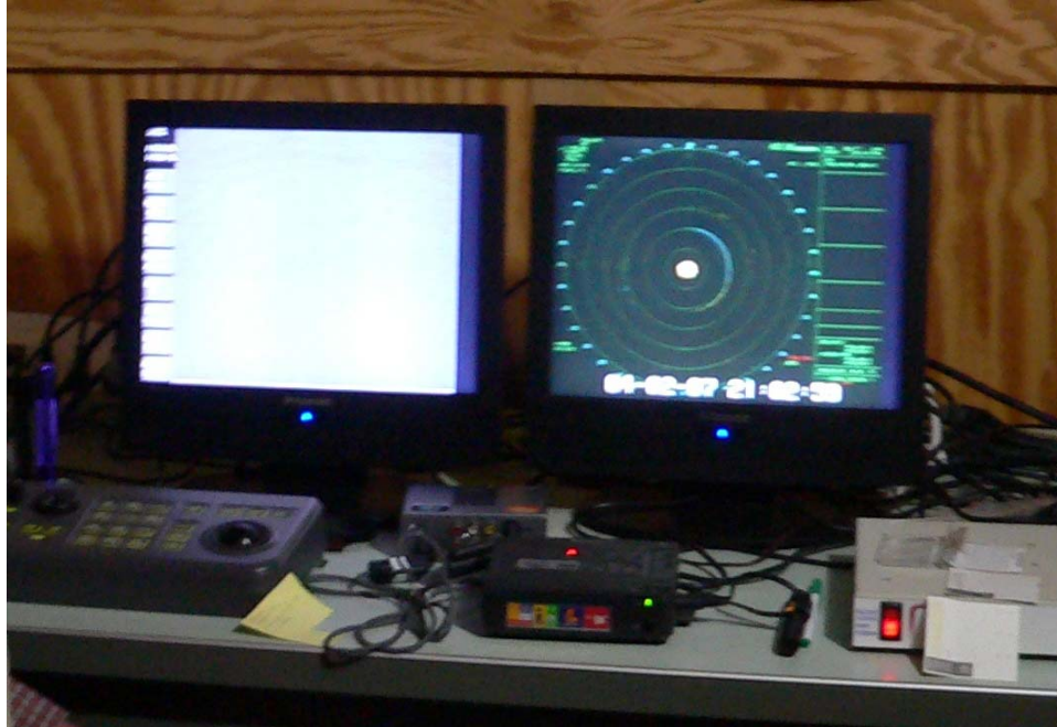
Figure 6-9. Dual display of video from thermal imager (left) and vertically-pointing radar (right).
