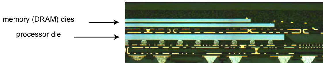
Figure 33: Apple A4 processor cross-section.
