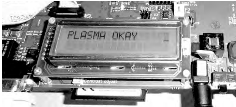
Figure 36: Example of FPGA-based checker failure reporting during our developmental testing, using the Plasma processor model from OpenCores.
