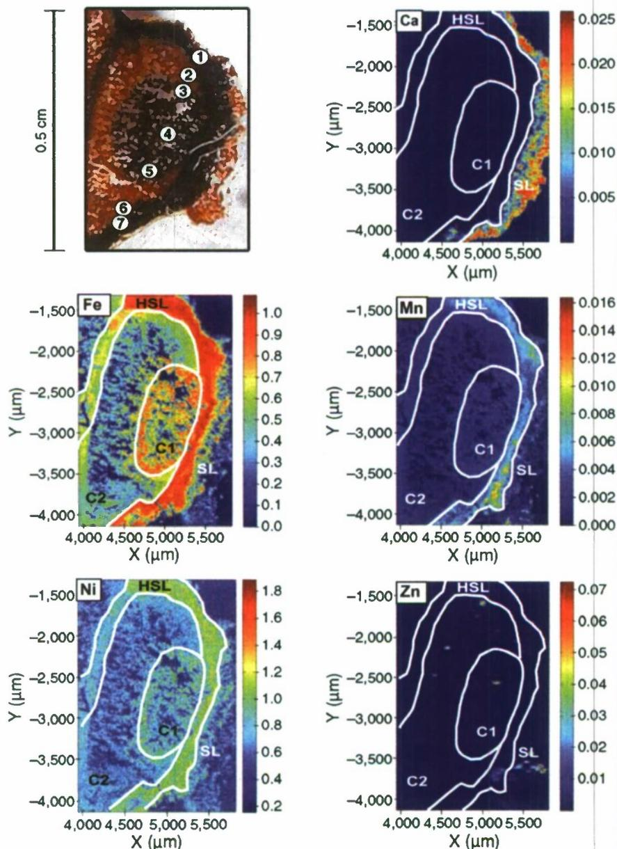
**FIGURE 5.**  $\mu$ -XRF maps of Ca, Fe, Mn, Ni, and Zn concentrations for a representative micro-sized tube shaped iron corrosion product. The numbers indicate the locations of the representative  $\mu$ -XRD traces. Core (C), hard shell layer (HSL), surface layer (SL).
