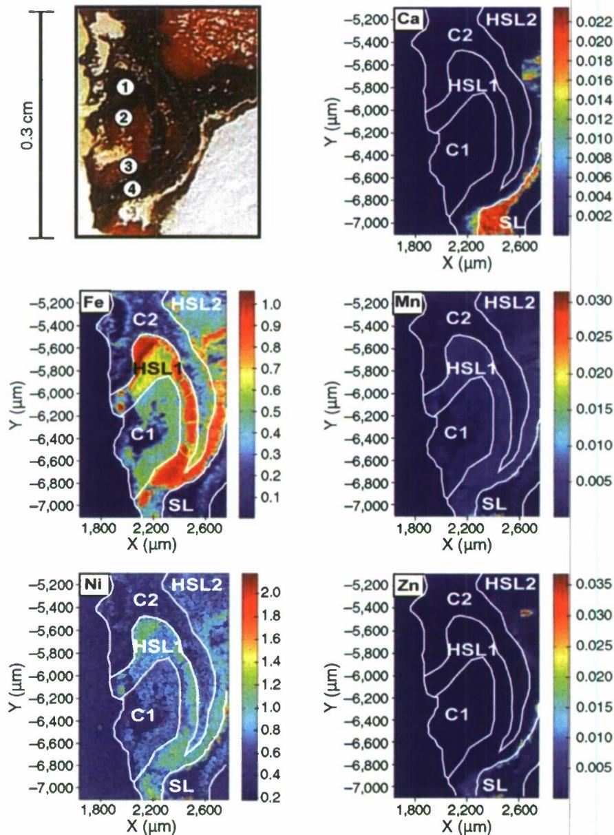
**FIGURE 4.**  $\mu$ -XRF maps of Ca, Fe, Mn, Ni, and Zn concentrations for a micro-sized classic mound-shaped iron corrosion product. The numbers indicate the locations of the representative  $\mu$ -XRD traces. Core (C), hard shell layer (HSL), surface layer (SL).
