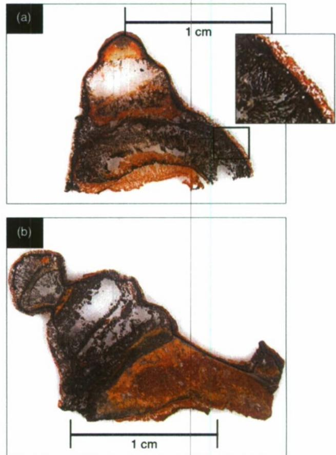
**FIGURE 2.** Cross sections of corrosion products mounted on quartz slides and polished to an average thickness of 35  $\mu\text{m}$ : (a) free-standing tube cut parallel to the long axis and (b) mound with tube cut parallel to the long axis of the tube. Enlargement showing details of HSL and SL uniformly encasing corrosion products.
