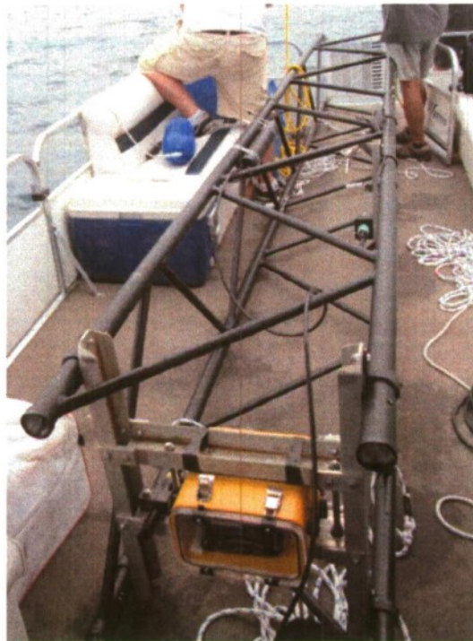
Figure 3. Picture of IMAST during SOTEX deployment. Notice the camera in the housing (bottom of the picture) and passive resolution target at the far end of the IMAST.
