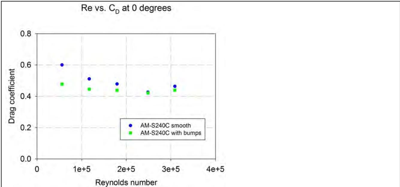
Fig. 8. Water tunnel results with tag AM-240C. Drag coefficient as a function of Reynolds number at the  $0^\circ$  orientation.
