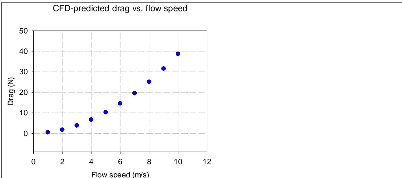
Fig. 7. SolidWorks CFD predictions of drag (Newtons) vs. flow speed (m/s).
