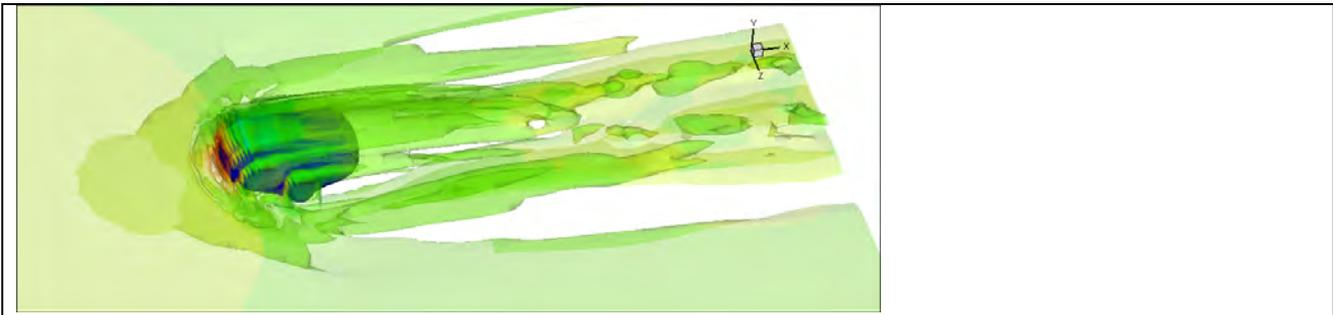
Fig. 1. Vortex structures computed for the new tag (AM-240C) with zero gap and zero inclination.
