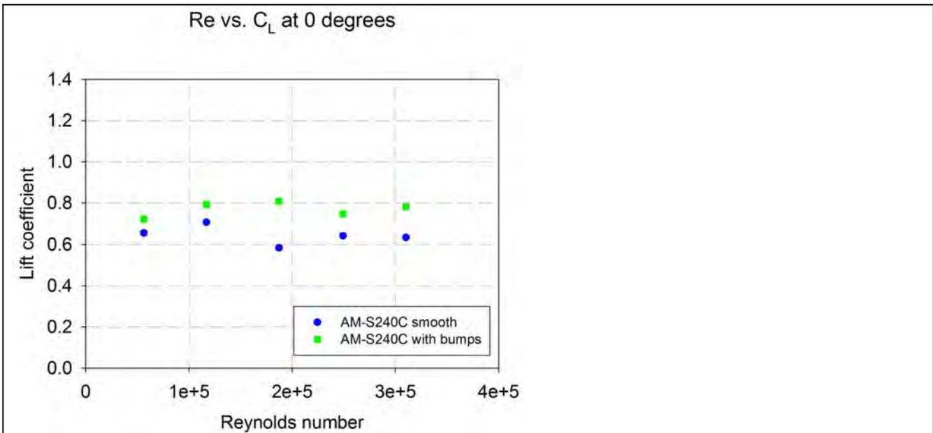
Fig. 9. Water tunnel results with tag AM-240C. Lift coefficient as a function of Reynolds number at the  $0^\circ$  flow orientation.
