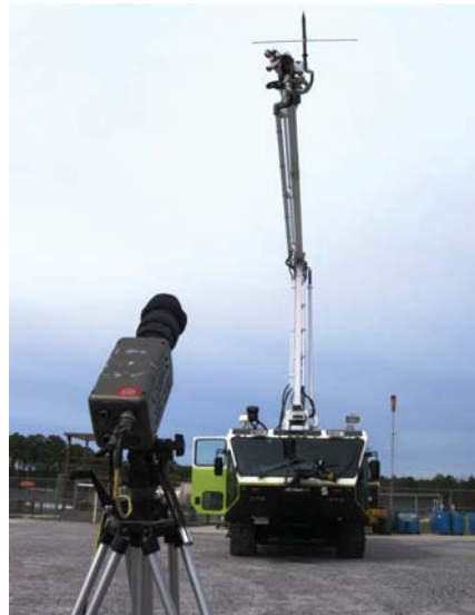
Figure 38. Typical Test Setting for Boom Oscillation Tests
