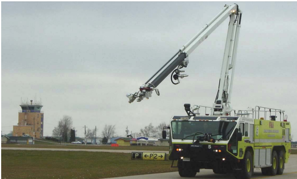
Figure 1. The FAA Striker With Deployed HRET
