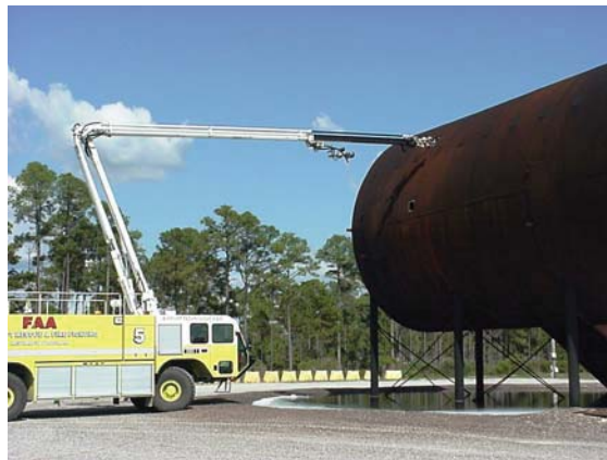
Figure 35. Penetrating the Upper Passenger Deck
