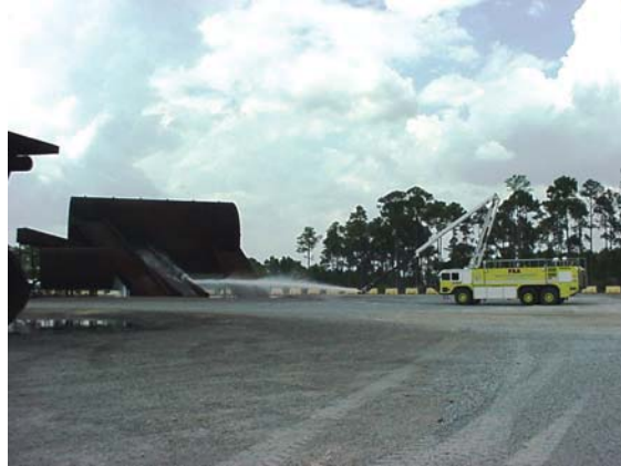
Figure 56. Tip Turret Initial Attack
