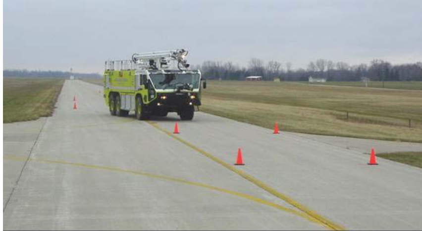
Figure 17. The FAA Striker HRET During NATO Lane Change Test
