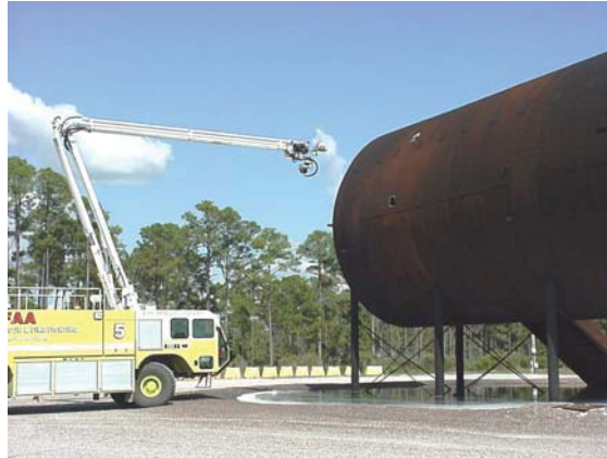
Figure 34. Extending the Boom for High Attack
