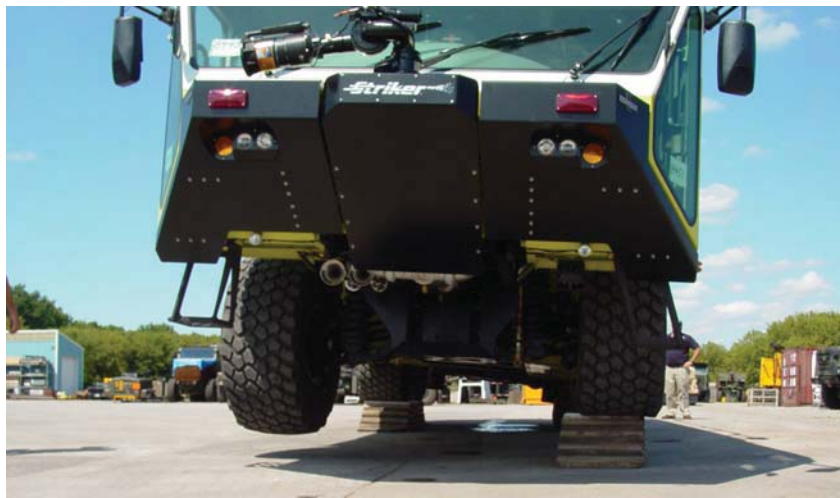
Figure 12. The FAA Striker Baseline Chassis Flexibility Test
