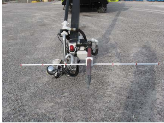
Figure 37. Distance Reference for Measuring Oscillation Magnitude
