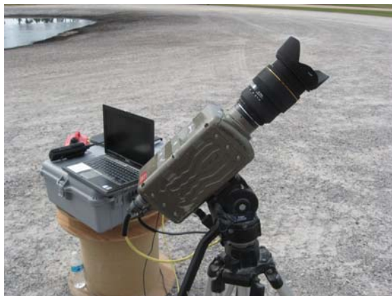
Figure 36. High-Speed Camera and Data Computer
