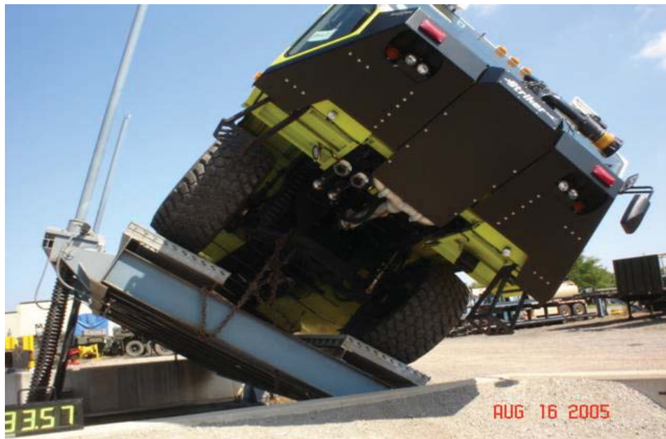
Figure 6. Tilt Table Test Without the HRET
