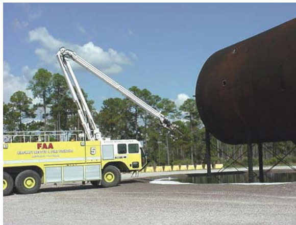
Figure 31. Extending the Lower Boom for low Attack
