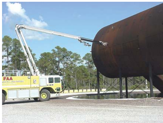
Figure 33. Penetrating the Lower Passenger Deck
