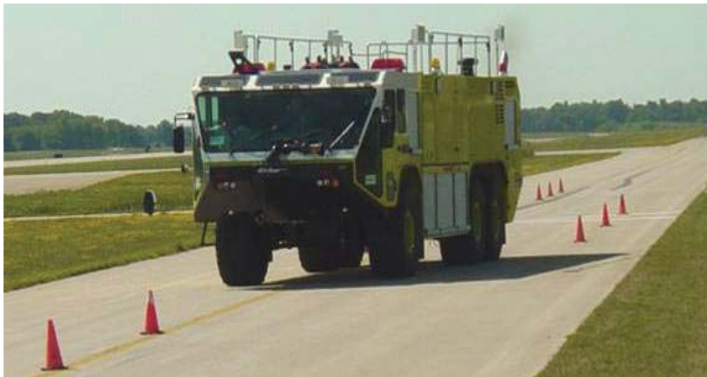
Figure 16. The FAA Striker Baseline During NATO Lane Change Test
