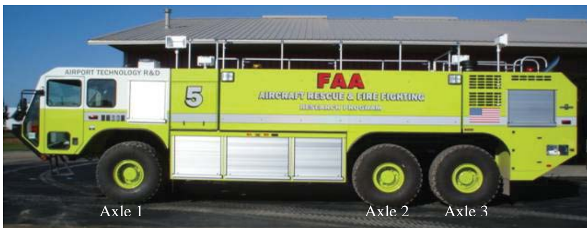
Figure 3. The FAA Striker 6X6 ARFF Vehicle Showing Axle Designations
