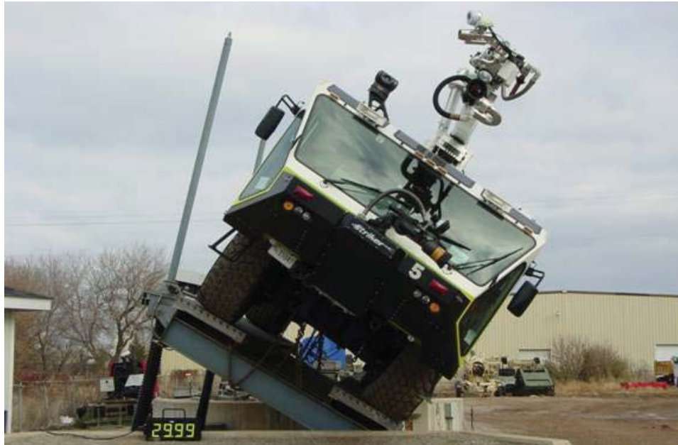
Figure 7. Tilt Table Test With the HRET
