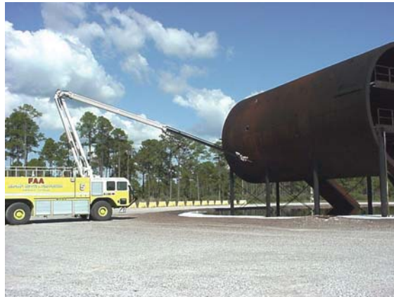
Figure 32. Penetrating the Cargo Deck
