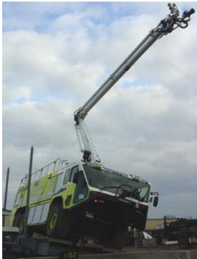
Figure 8. Tilt Table Test With the HRET Elevated
