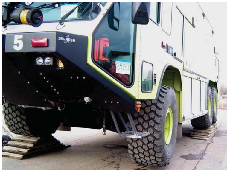
Figure 13. The FAA Striker HRET Chassis Flexibility Test
