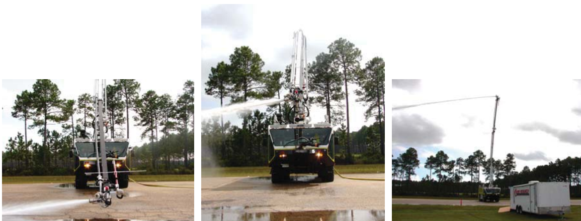
Figure 39. Oscillation Tests With Water Spray
