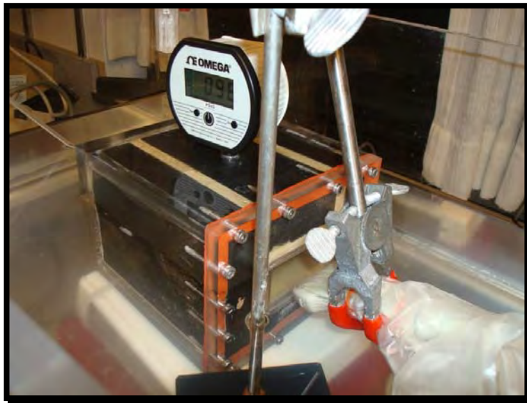
Figure 1. The re-designed water tank scanned by the L14-5 transducer. Notice the digital pressure gauge on the top of the tank.
