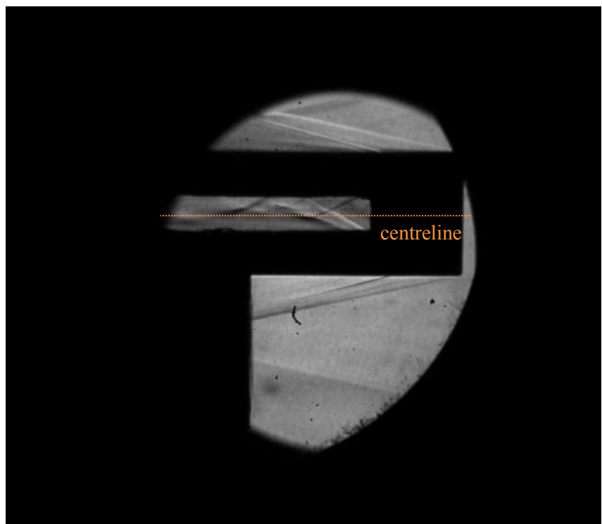
Figure 42: Schlieren snapshot at t = 1.302 seconds, with the difference in door edge shocks displayed by highlighting that the reflection point of the shocks does not lie on the centreline, but above
