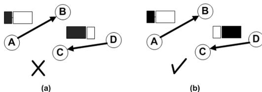
**Fig. 10.** An example to illustrate interference-aware bandwidth selection. The portion of bandwidth used by the transmissions is shaded black. A cross mark indicates that the transmissions cannot take place simultaneously and a check mark indicates that the two transmissions can be scheduled simultaneously.
