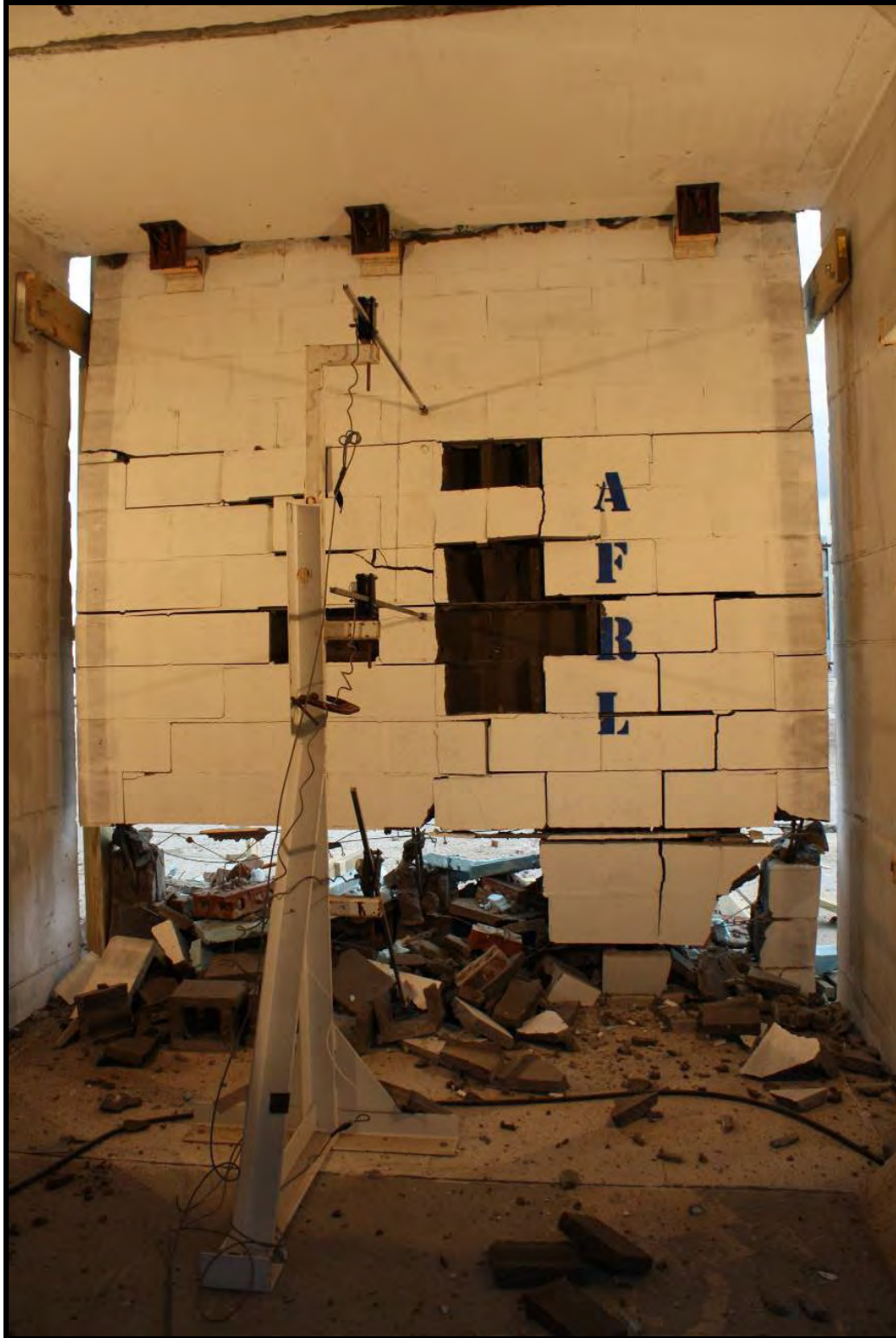
Figure C-40. Experiment 2 cavity wall panel full interior view
