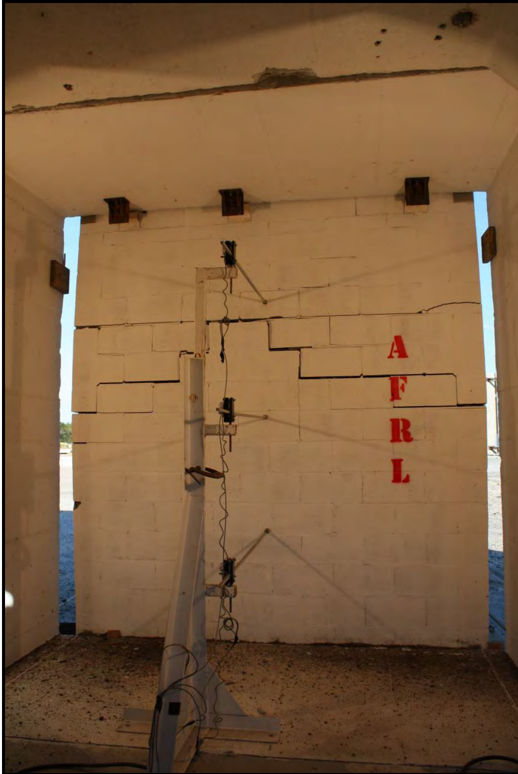
Figure C-17. Experiment 1 cavity wall panel full interior view
