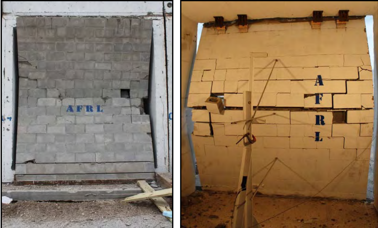
Figure 33. Experiment 2 Post-detonation 6-inch CMU Panel Exterior View (left) and Interior View (right)
