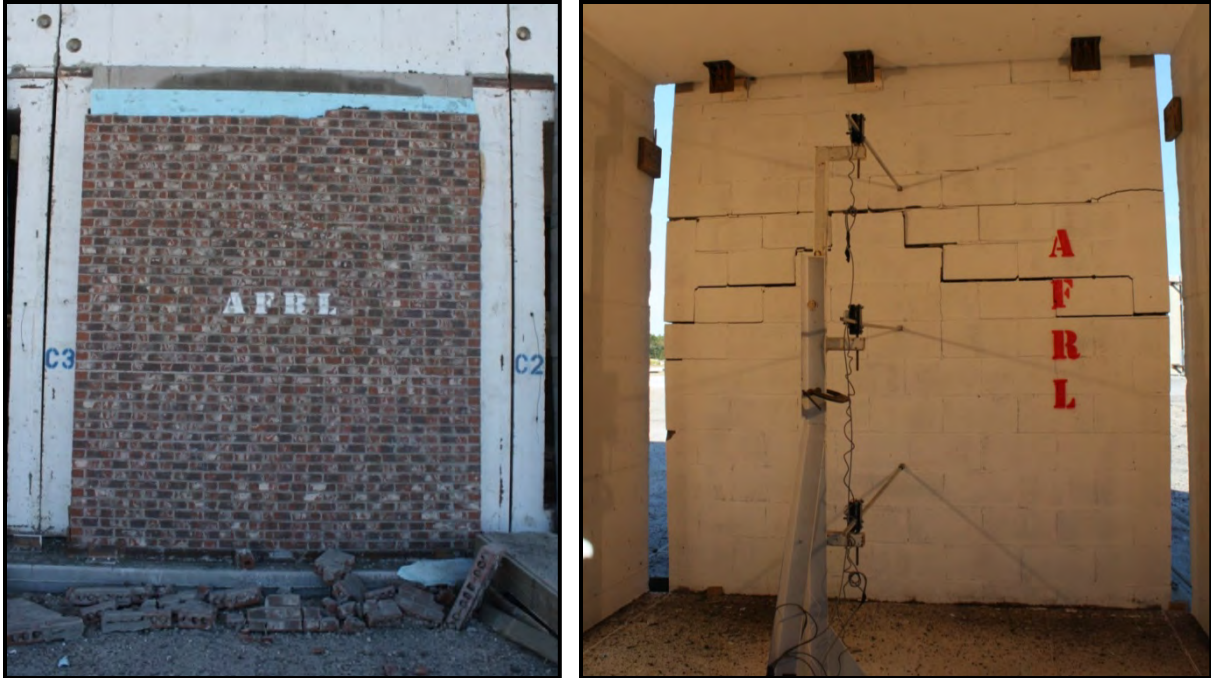
Figure 28. Experiment 1 Post-detonation Cavity Wall Exterior View (left) and Interior View (right)
