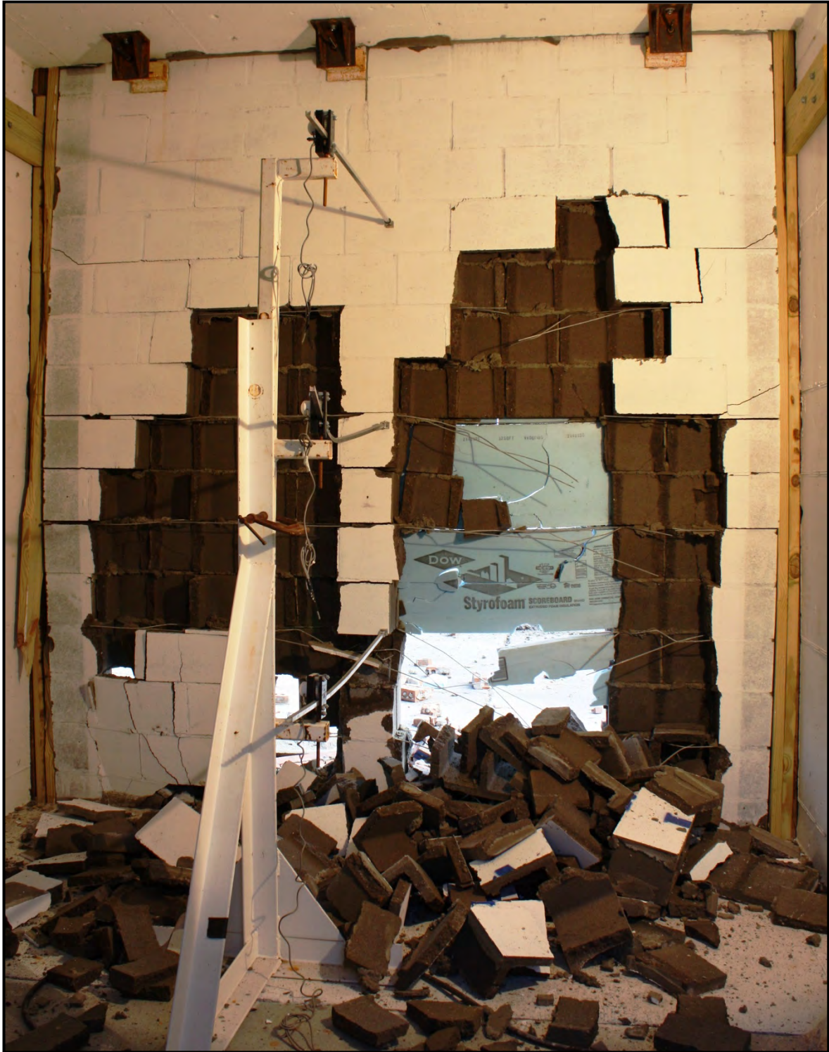
Figure C-65. Experiment 3 cavity wall panel full interior view
