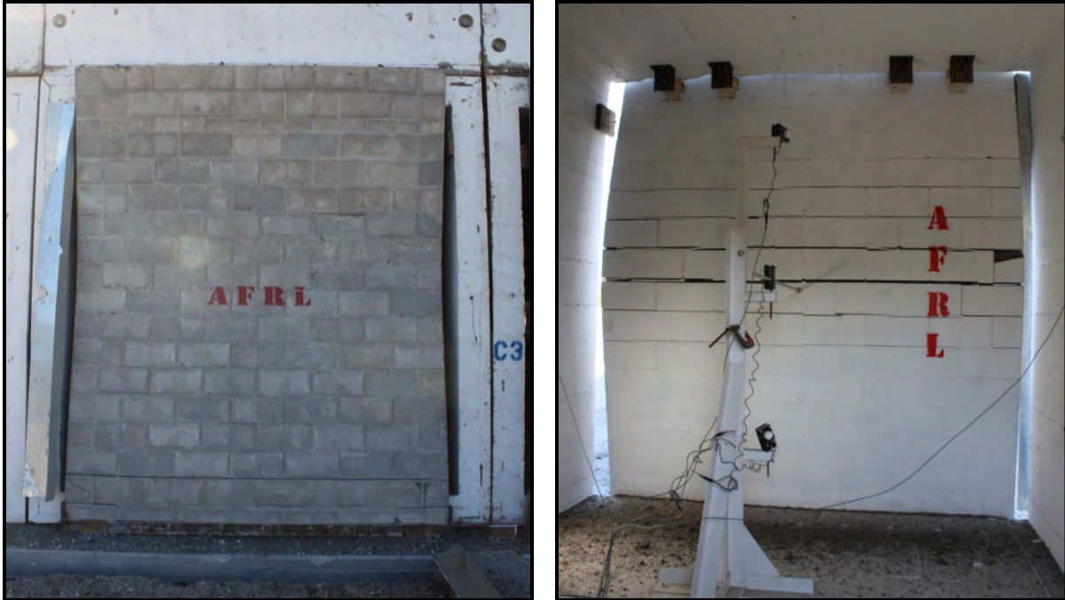
Figure 21. Experiment 1 Post-Detonation 6-inch CMU Panel Exterior View (left) and Interior View (right)
