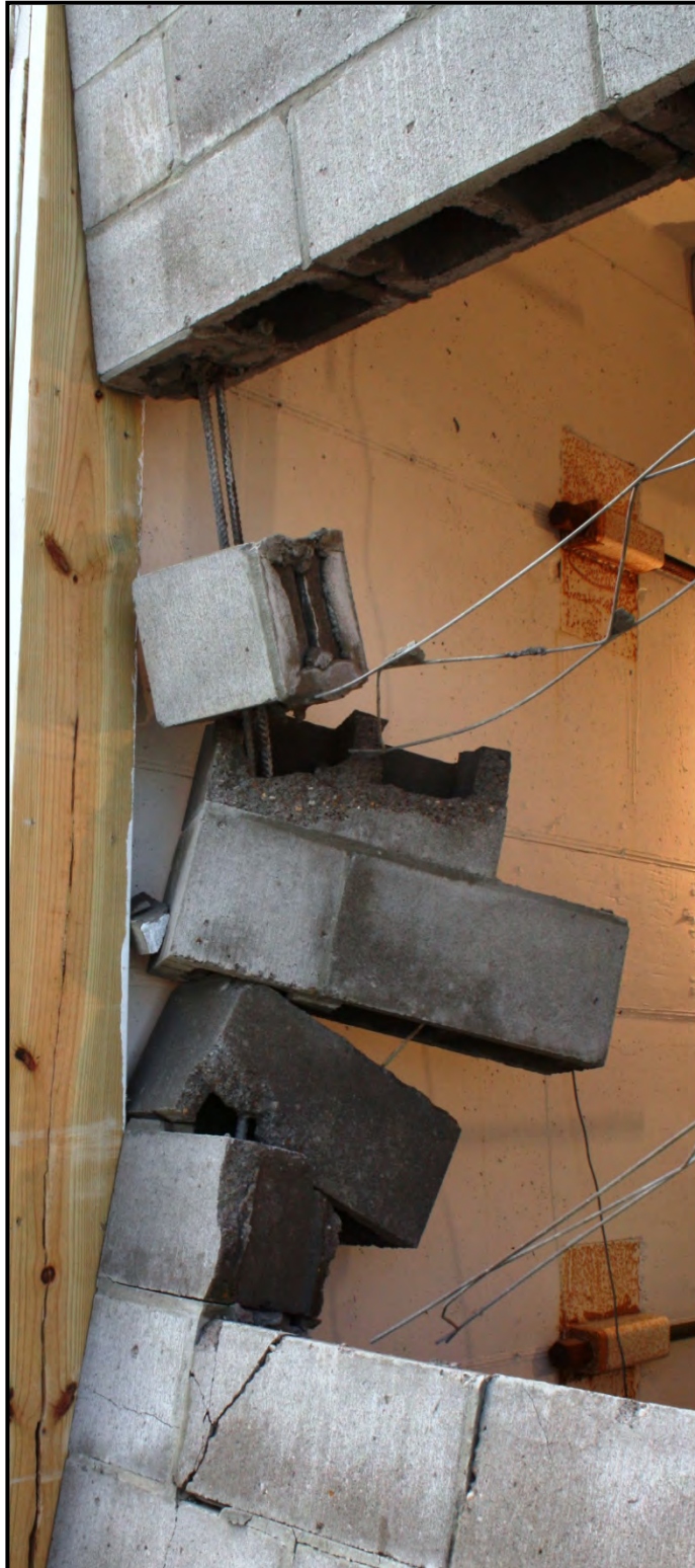
Figure C-51. Experiment 3 8-inch CMU panel breaching exterior view, improperly grouted reinforced cells
