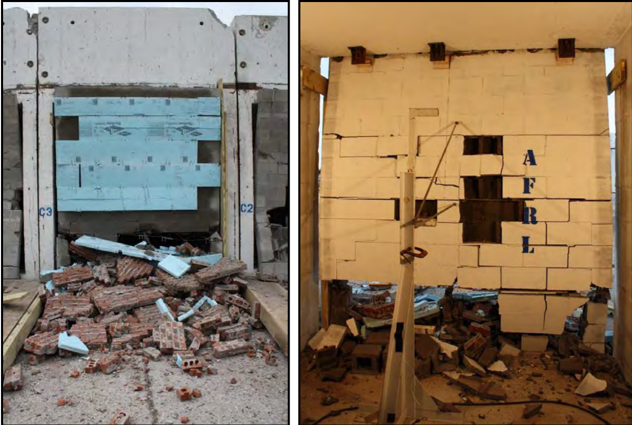
Figure 42. Experiment 2 Post-detonation Cavity Wall Exterior View (left) and Interior View (right)
