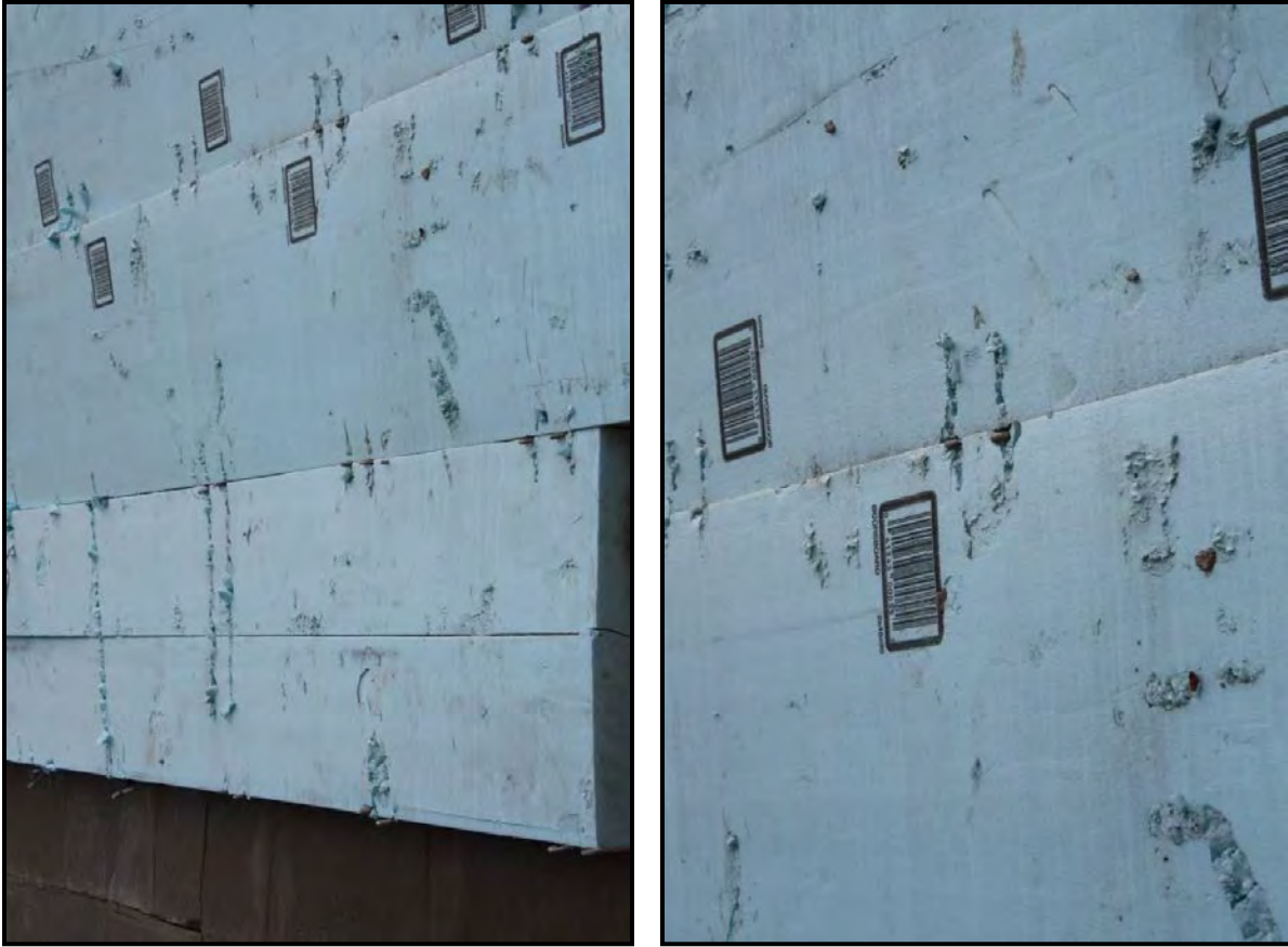
Figure 43. Experiment 2 Post-detonation Cavity Wall Foam Damage
