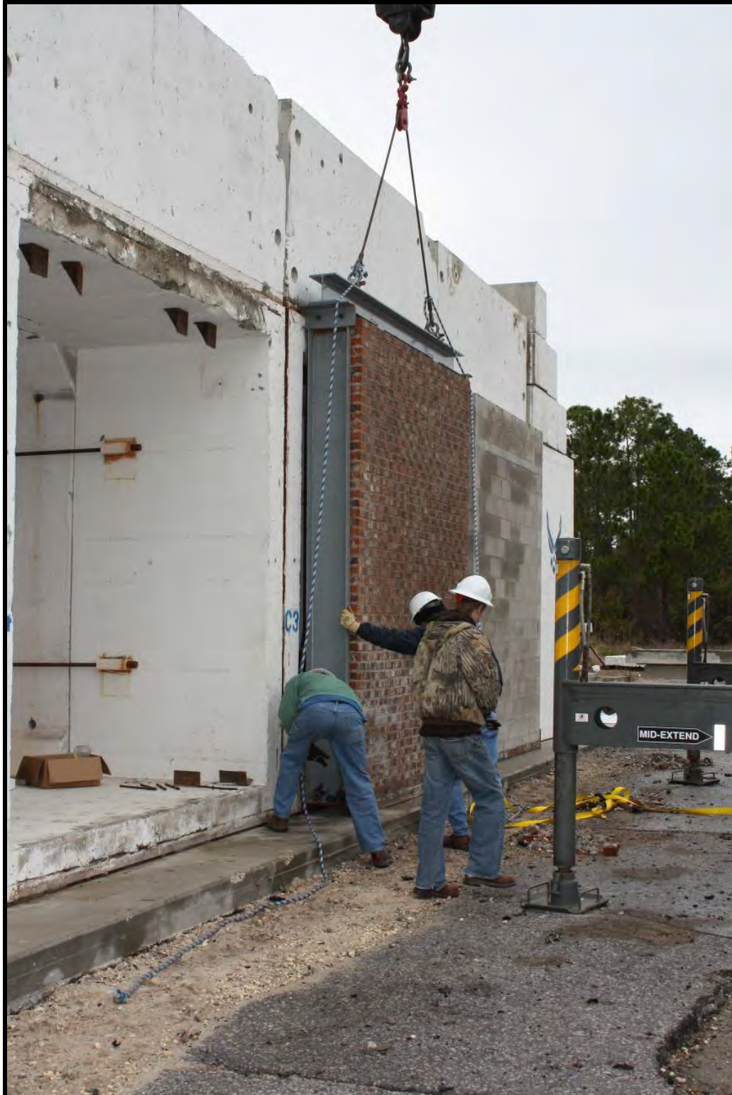
Figure B-53. Test panels being positioned for testing
