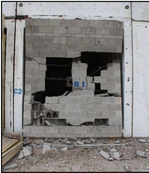
Figure 37. Experiment 2 Post-detonation 8-inch CMU Panel Exterior View (left) and Interior View (right)
