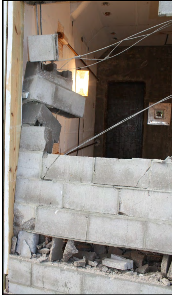
Figure 53. Experiment 3 Post-detonation 8-inch CMU Panel Close-up Exterior Views
