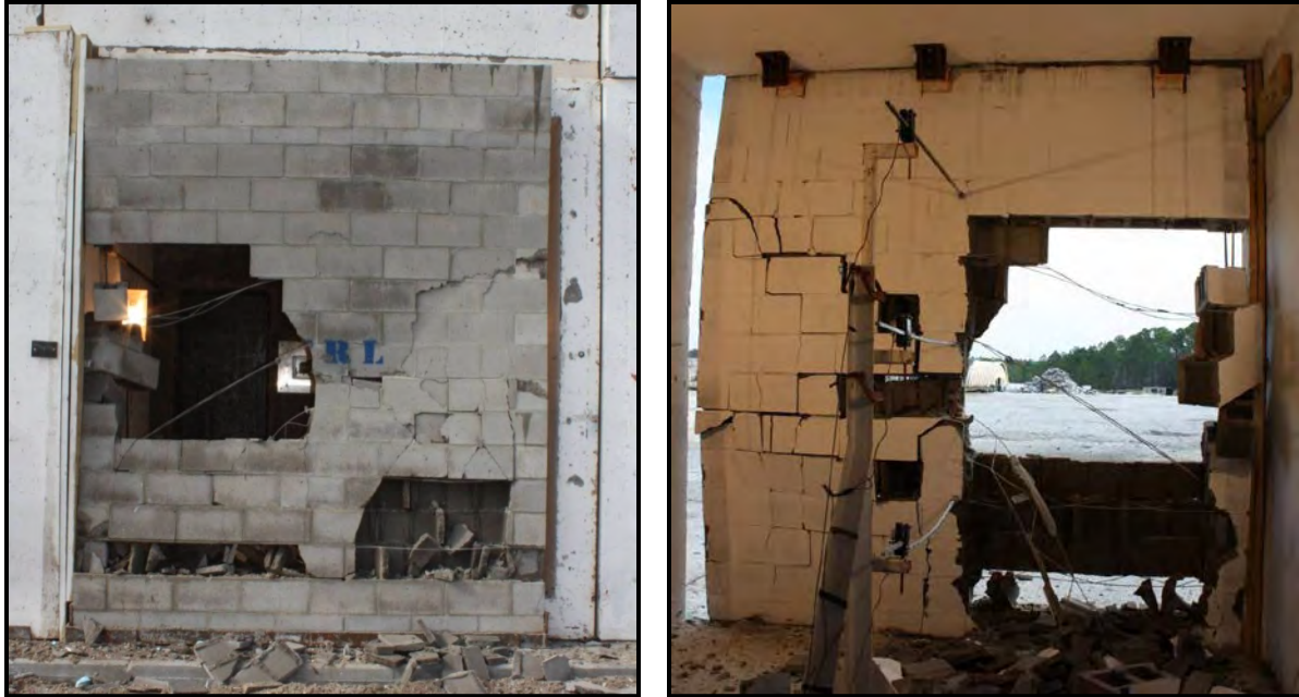
Figure 52. Experiment 3 Post-detonation 8-inch CMU Panel Exterior View (left) and Interior View (right)
