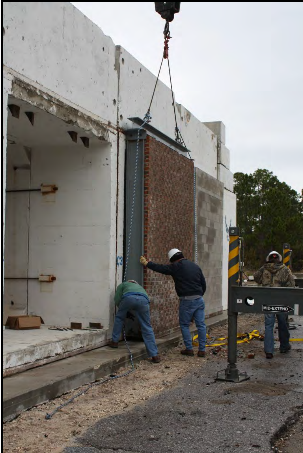
Figure B-54. Test panels being positioned for testing
