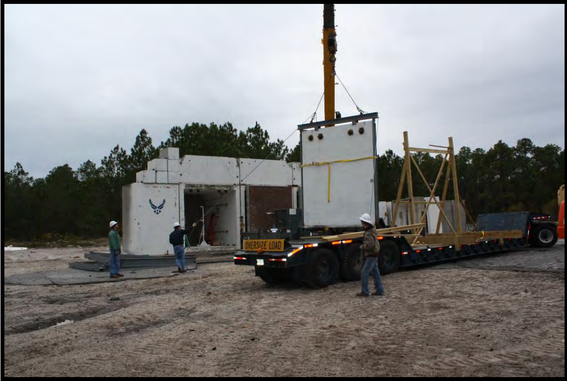
Figure B-61. Test panels being positioned for testing
