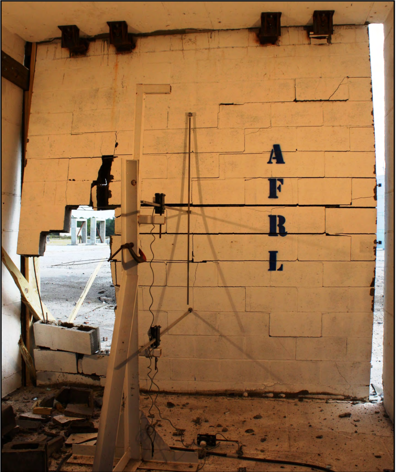
Figure C-48. Experiment 3 6-inch CMU panel full interior view
