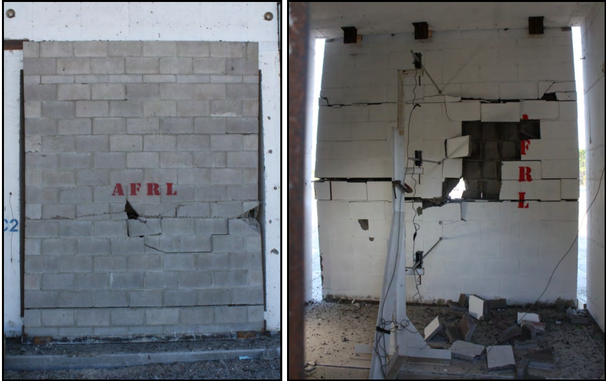
Figure 24. Experiment 1 Post-detonation 8-inch CMU Panel Exterior View (left) and Interior View (right)
