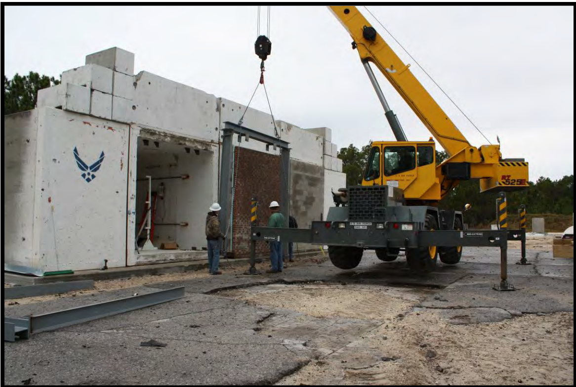
Figure B-56. Test panels being positioned for testing
