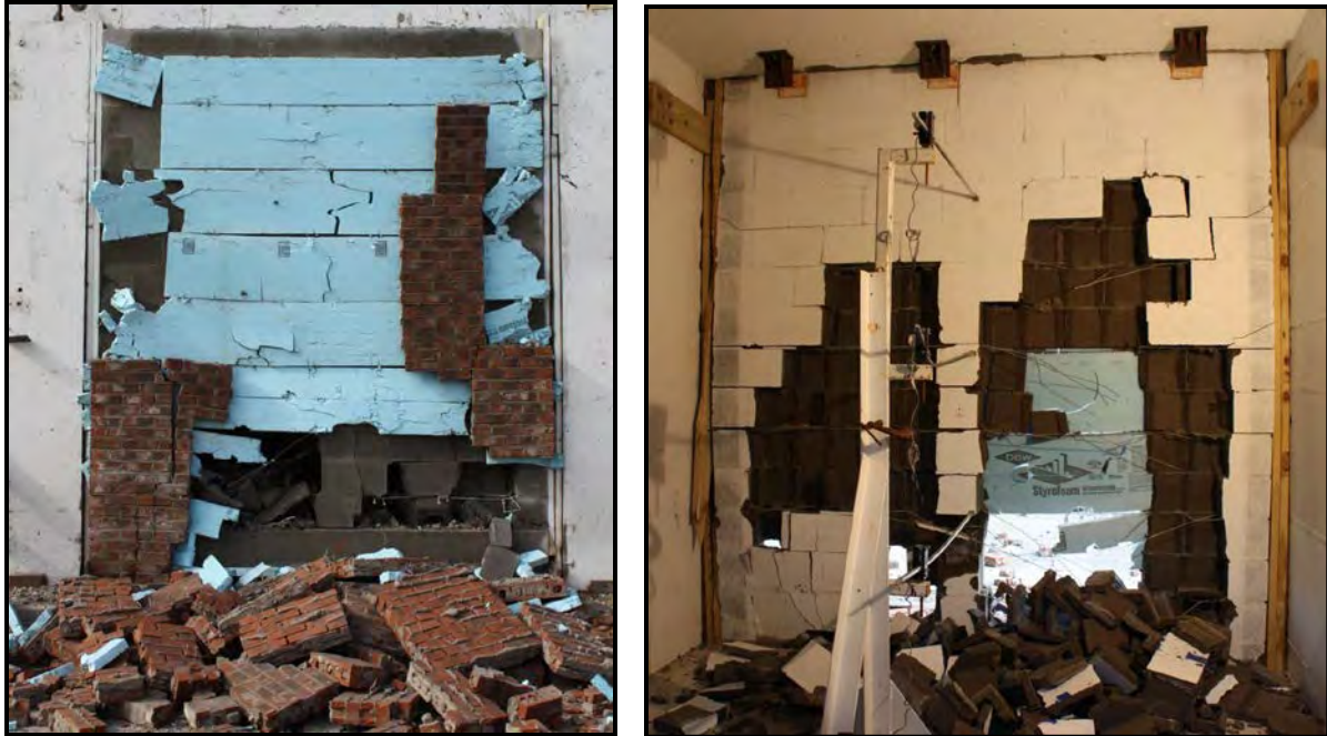
Figure 57. Experiment 3 Post-detonation Cavity Wall Exterior View (left) and Interior View (right)
