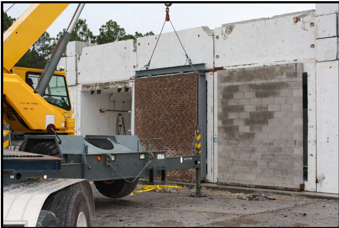
Figure B-52. Test panels being positioned for testing
