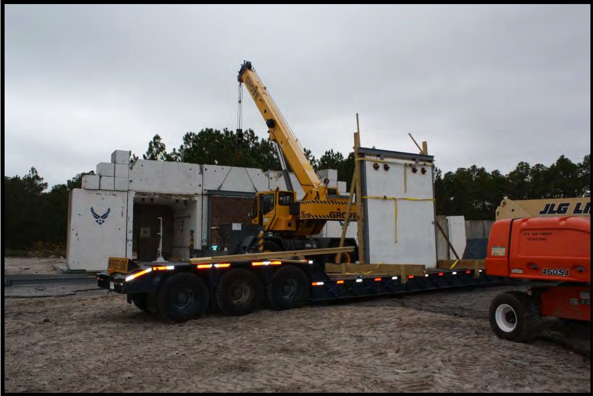
Figure B-49. Test panels being positioned for testing
