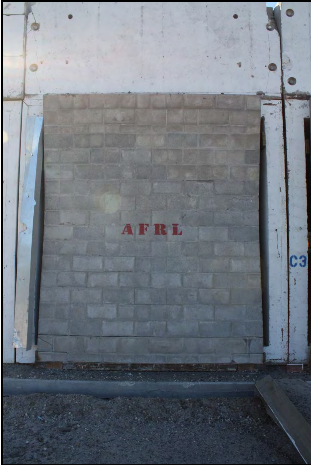
Figure C-6. Experiment 1 6-inch CMU panel front view
