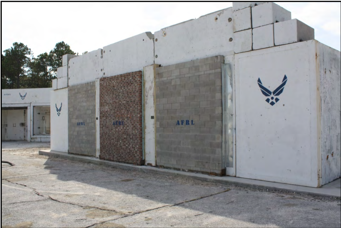
Figure 12. Panels in Reaction Structure Ready for Testing
