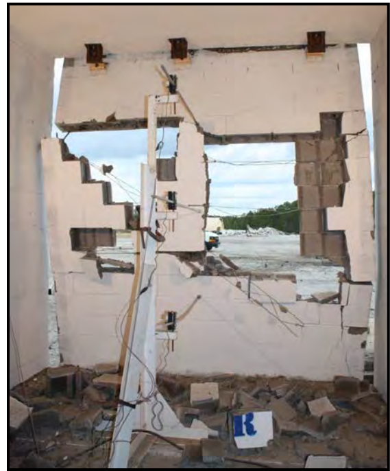
Figure 37. Experiment 2 Post-detonation 8-inch CMU Panel Exterior View (left) and Interior View (right)
