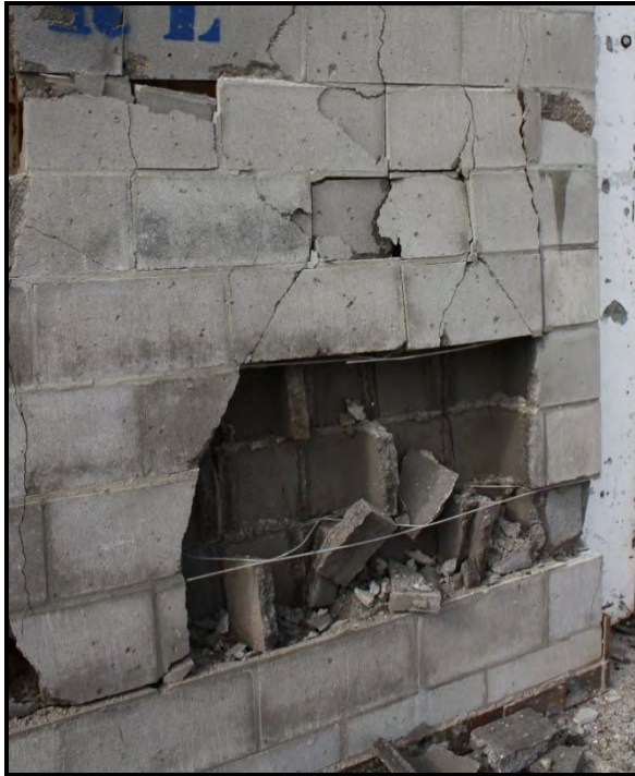
Figure 53. Experiment 3 Post-detonation 8-inch CMU Panel Close-up Exterior Views
