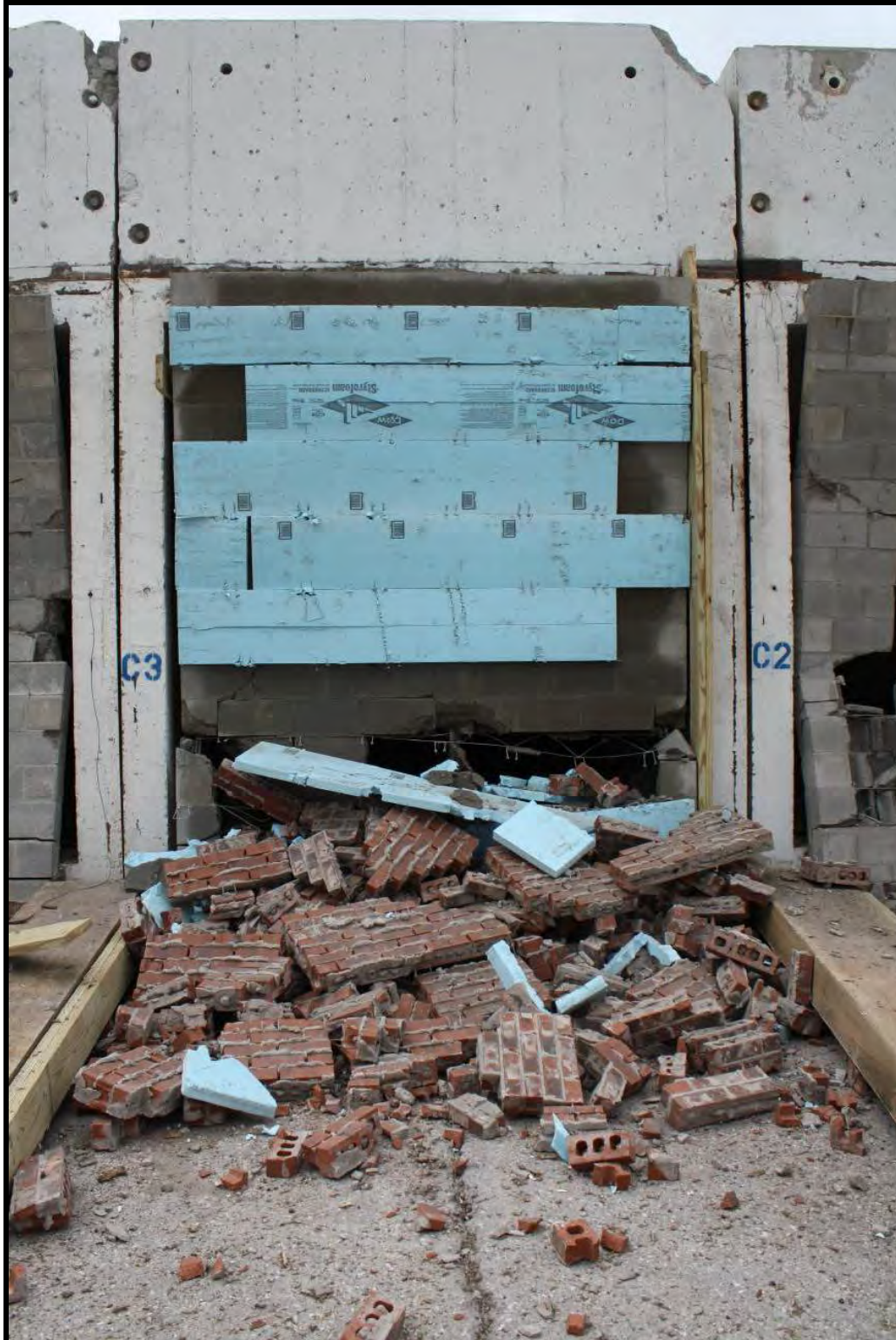
Figure C-35. Experiment 2 cavity wall panel front view
