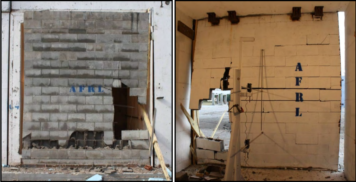
Figure 48. Experiment 3 Post-detonation 6-inch CMU Panel Exterior View (left) and Interior View (right)
