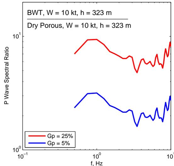
**Figure 7. Spectral ratios of the estimated station MNV P wave spectrum for a 10 kt explosion at a depth of 323 m in saturated tuff to the corresponding MNV predicted spectra for 10 kt explosions in dry, porous media characterized by  $G_p$  values of 5% and 25%.**
