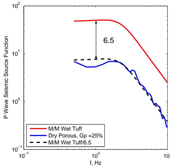
Figure 8. Comparison of the P wave source function estimate for a 10 kt explosion at a depth of 323 m in a dry, porous medium characterized by a  $G_p$  value of 25% with the corresponding Mueller/Murphy source function for the same explosion in saturated tuff.
