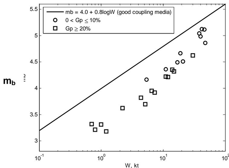
**Figure 1. Comparison of observed  $m_b$ /yield data for explosions conducted in dry, porous tuff and alluvium above the water table at NNSS with the nominal NNSS  $m_b$ /yield relation for explosions conducted in good-coupling media.  $G_p$  denotes the measured air-filled porosity (percent by volume) at the detonation point.**
