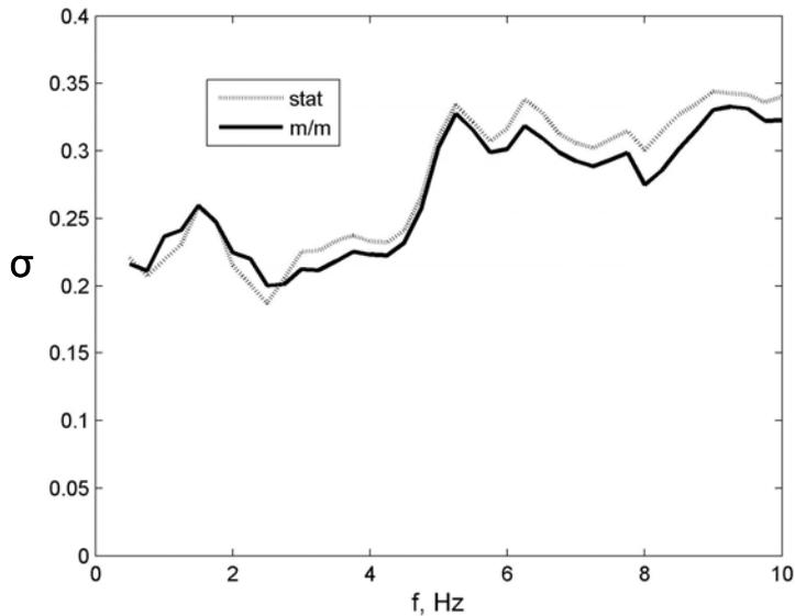
Figure 9. Comparison of prediction standard deviations ( $\sigma$ ) as a function of frequency obtained using the statistical yield scaling model (stat) and the Mueller/Murphy (m/m) yield and depth scaling model for explosions in saturated tuff, evaluated over all explosions in the selected dry, porous sample and with yields less than or equal to 20 kt.
