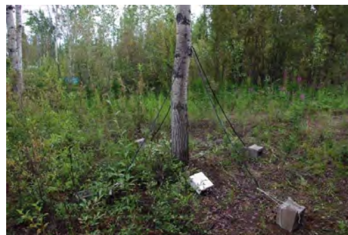
Figure 45: Photograph of the ELF/VLF receiver installed at Tok, AK
