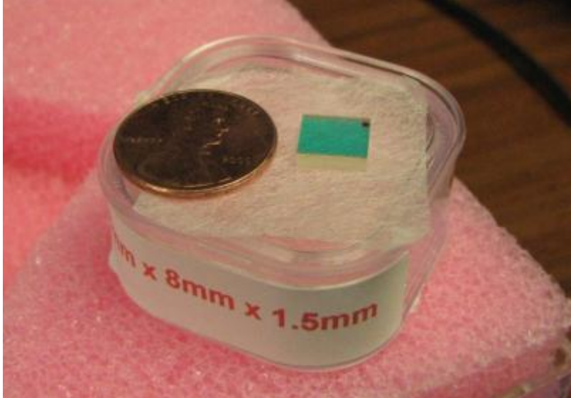
Figure 23: Photo of Tm:YAG crystal, 6% doping, 1.5 mm thick, AR coated.
