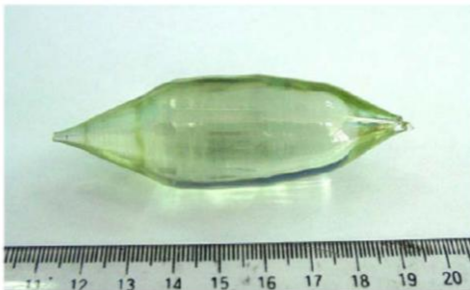
Figure 11: Photograph of bulk \text{Tm}:\text{YAG} crystal grown by Czochralski method [23].
