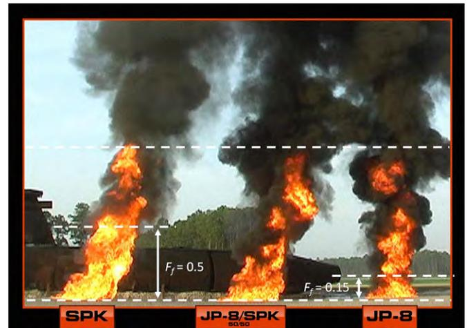
Fig. 1. Comparison of smoke properties for JP-8, SPK (S-8), and SPK/JP-8 blend including estimates of flame fraction ( $F_f$ ).
