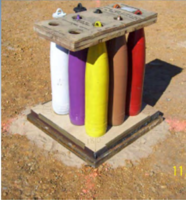
Test Setup Un-Confined Sympathetic Detonation Test
