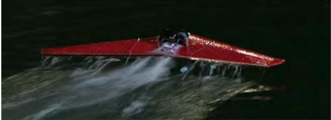
**Figure 27: Model trials showing trailing edge clearance and spray levels**
