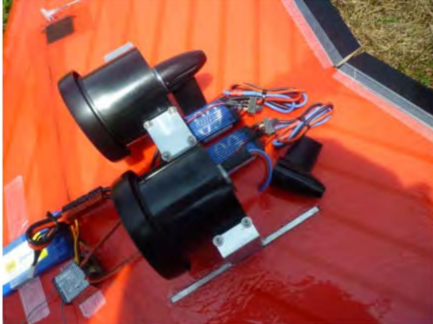
**Figure 24: Model arrangement of speed controllers, receiver, battery and ducted fans**
