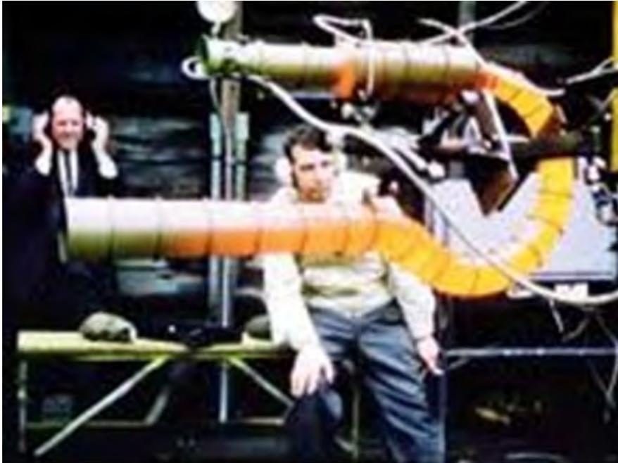
**Figure 3: Valve-less pulse jet on test bed<sup>3</sup>**
