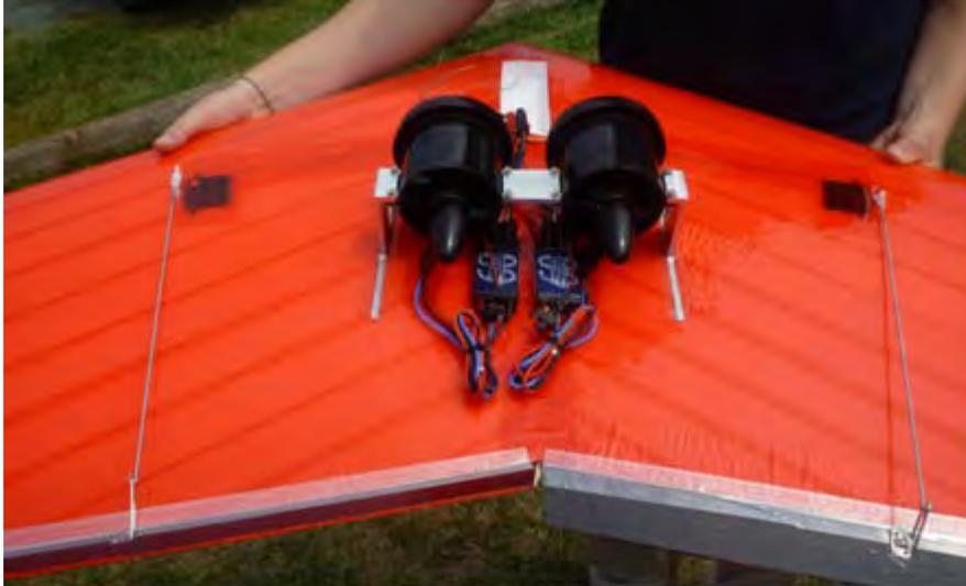
**Figure 25: Model elevon arrangement showing servo mounting and linkage**
