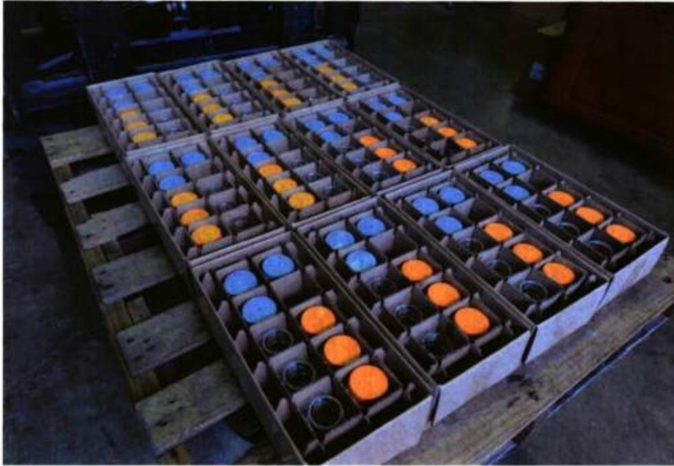
**Figure 2.7.20 Samples loaded on pallet to be exposed outdoors**
