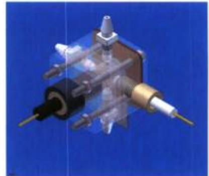
Figure 1.2.10 The modular stack cell
