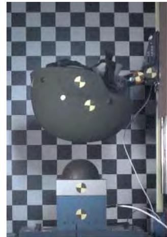
Figure 1: An ACH blunt impact evaluation in the crown impact location on the monorail drop tower.
