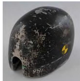
Figure 2: The DOT size “C” headform is the military standard for blunt impact testing of the size large ACH.
