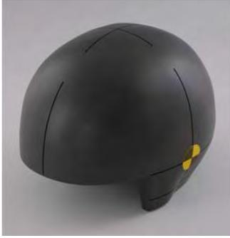
Figure 3: The ISO size “M” headform (used to fit the large ACH) is the standard for blunt impact testing of bicycle and motorcycle helmets.
