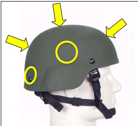
Figure 4: Helmet impact sites are highlighted for the Crown, Front, Right, Rear, and Right nape locations. Left and Left nape locations are symmetric to the Right.
