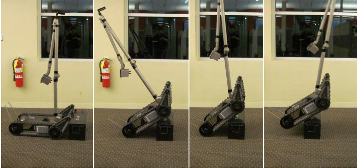
Figure 15: PackBot climbs over obstacle using active weight shifting
