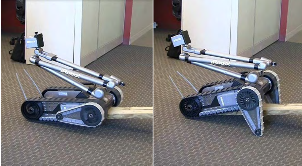
Figure 13: PackBot becomes high-centered on obstacle and spins its tracks in the air (left), High-centering prevention behavior uses flippers to free PackBot (right)
