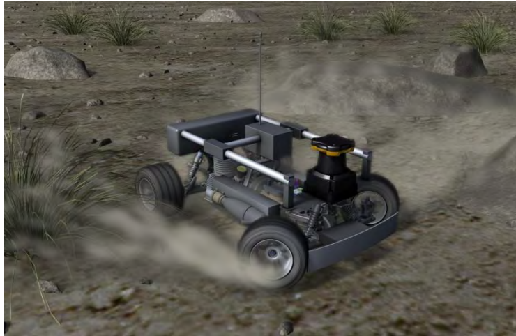
Figure 17: Dynamo high-speed small UGV hardware platform
