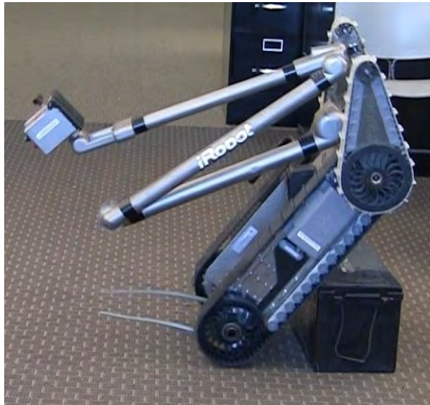
Figure 11: PackBot attempts to climb a tall obstacle and begins to roll over backwards
