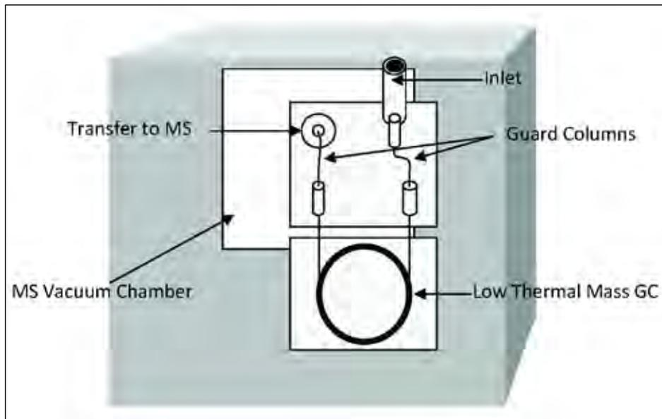
Figure 2.1. Components of the Griffin 450 GC-MS.
