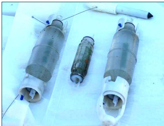
Figure 10. Snap Sampler samples showing black particles and piece of rusted casing (inside VOA vial).
