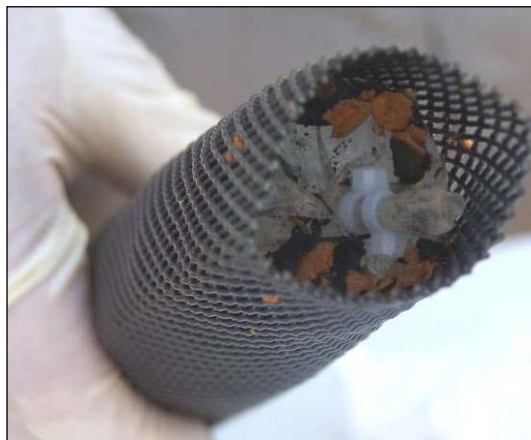
Figure 11. Top of RGC sampler showing deposits of large black and orange particles.
