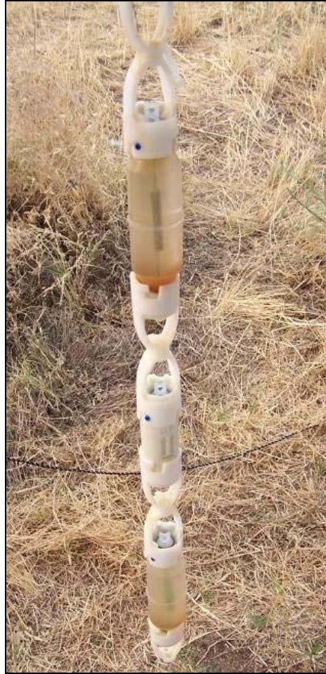
Figure 12. Snap Samplers containing an orange precipitate.
