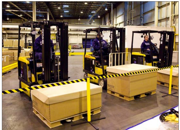
MHE POWERED BY FUEL CELLS, DLA DISTRIBUTION SUSQUEHANNA, PA COURTESY OF DEFENSE LOGISTICS AGENCY
