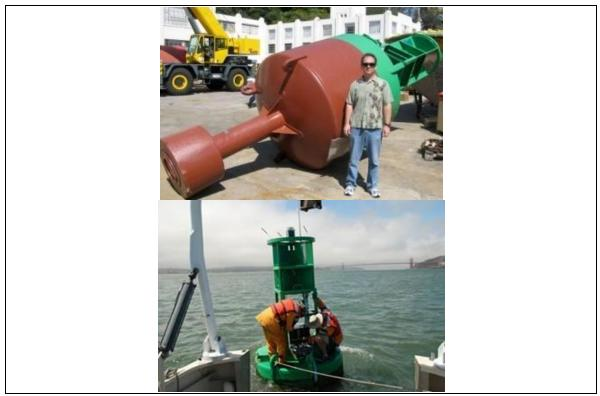
Figure 38. A Racom gateway kit with telesonar acoustic modem and cellular telephone modem implemented on a USCG navigation buoy in San Francisco Bay with logistical support by USCG cutter GEORGE COBB.
