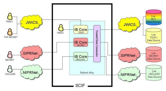
Figure 18. Proposed Radiant Alloy MDA system architecture
