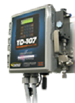
TD-107 Oil Content Monitors includes standard alarm relays, 4-20 mA output for remote monitoring, and a user-friendly USB data port for review of recorded discharge levels prior to port state control visits.
