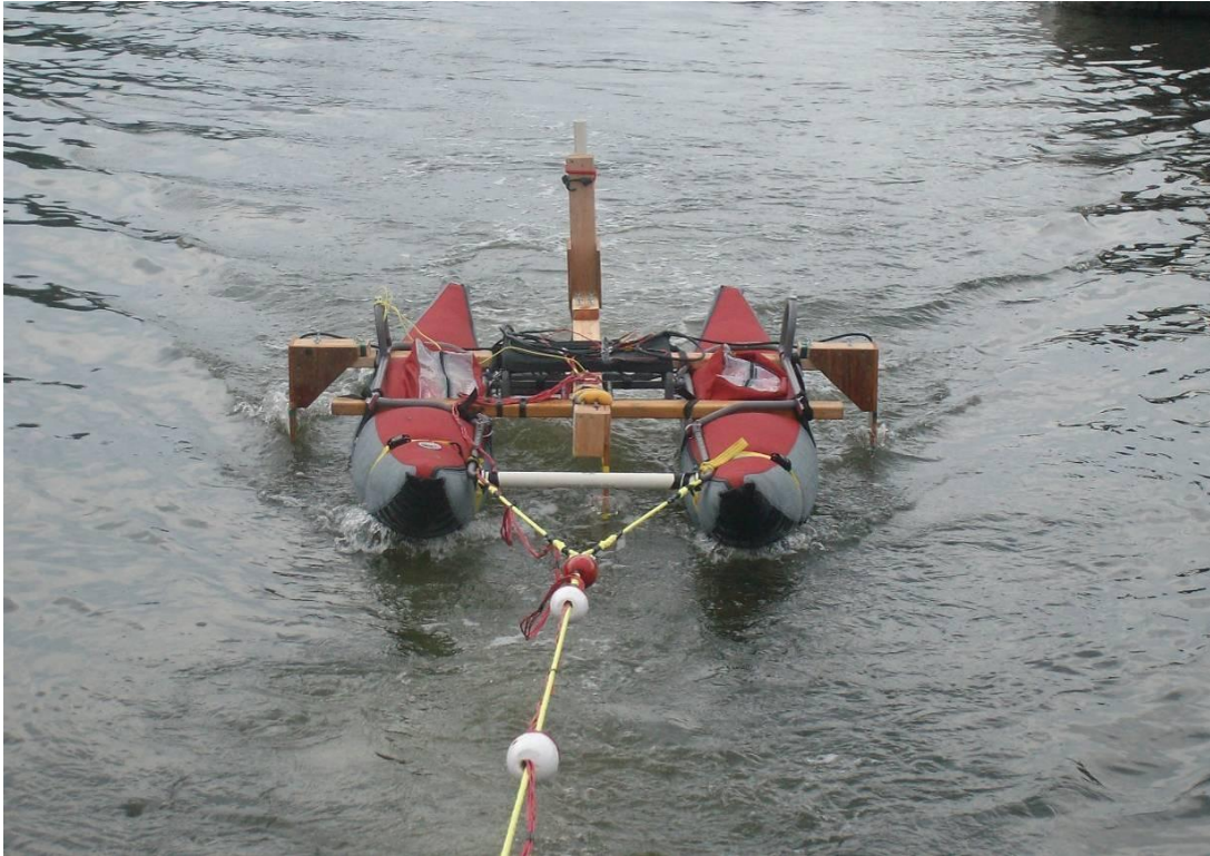
Figure 6. Free-field towed array apparatus during tow.
