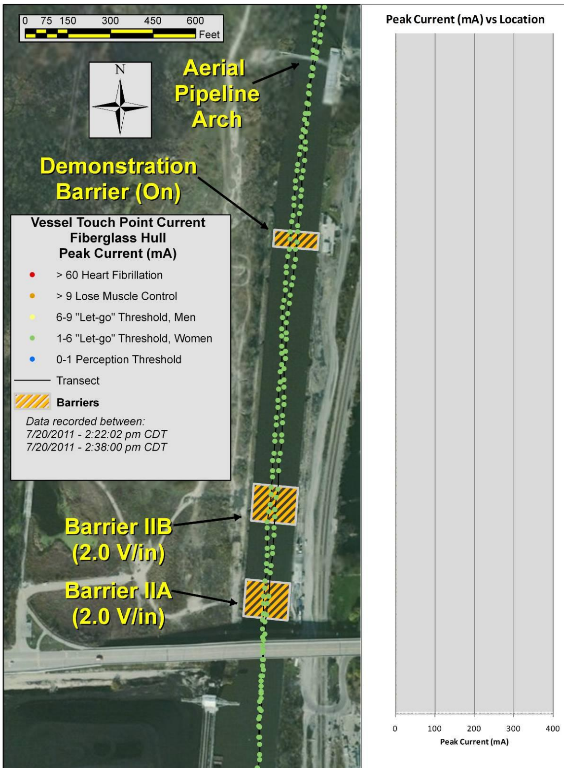
Figure 20. Peak rescue vessel electrical current (mA), fiberglass hull, 2.0 volts/inch.
