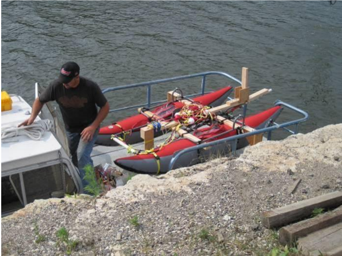
Figure 2. Towed free-field sensor array apparatus loaded on test vessel.
