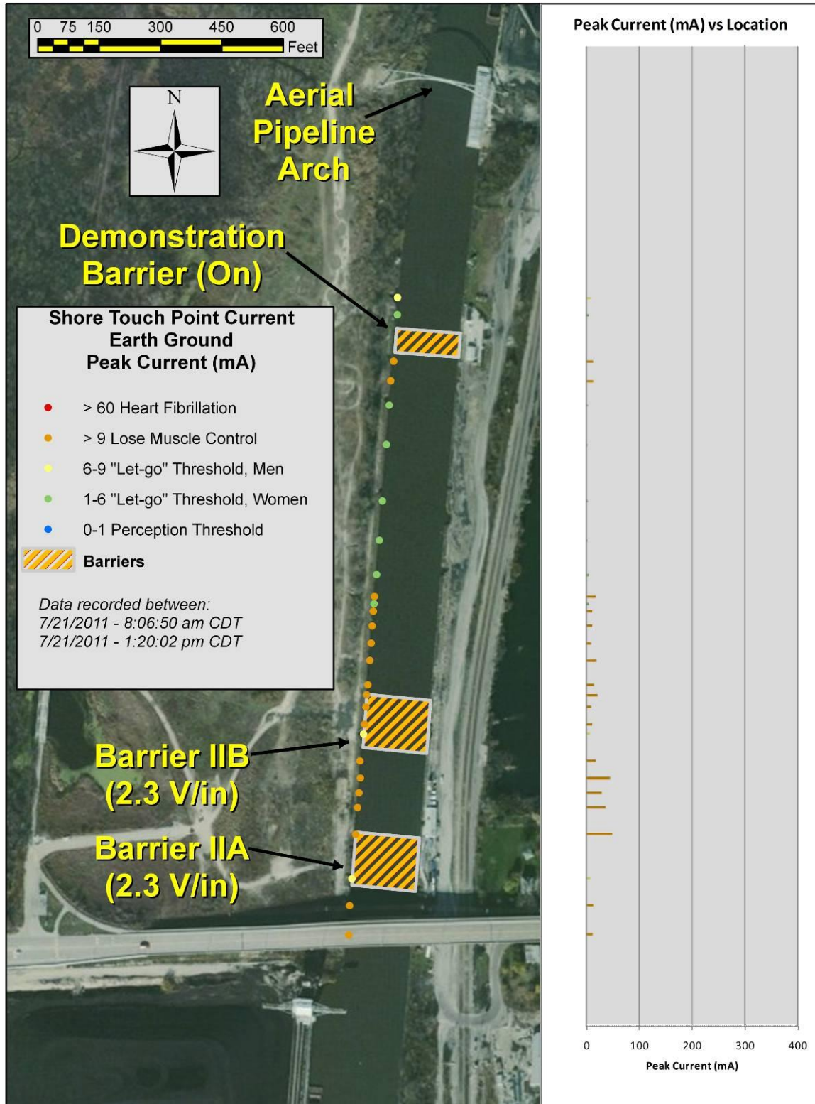
Figure 22. Results for shore touch-point current, “earth ground”, all barriers operating.
