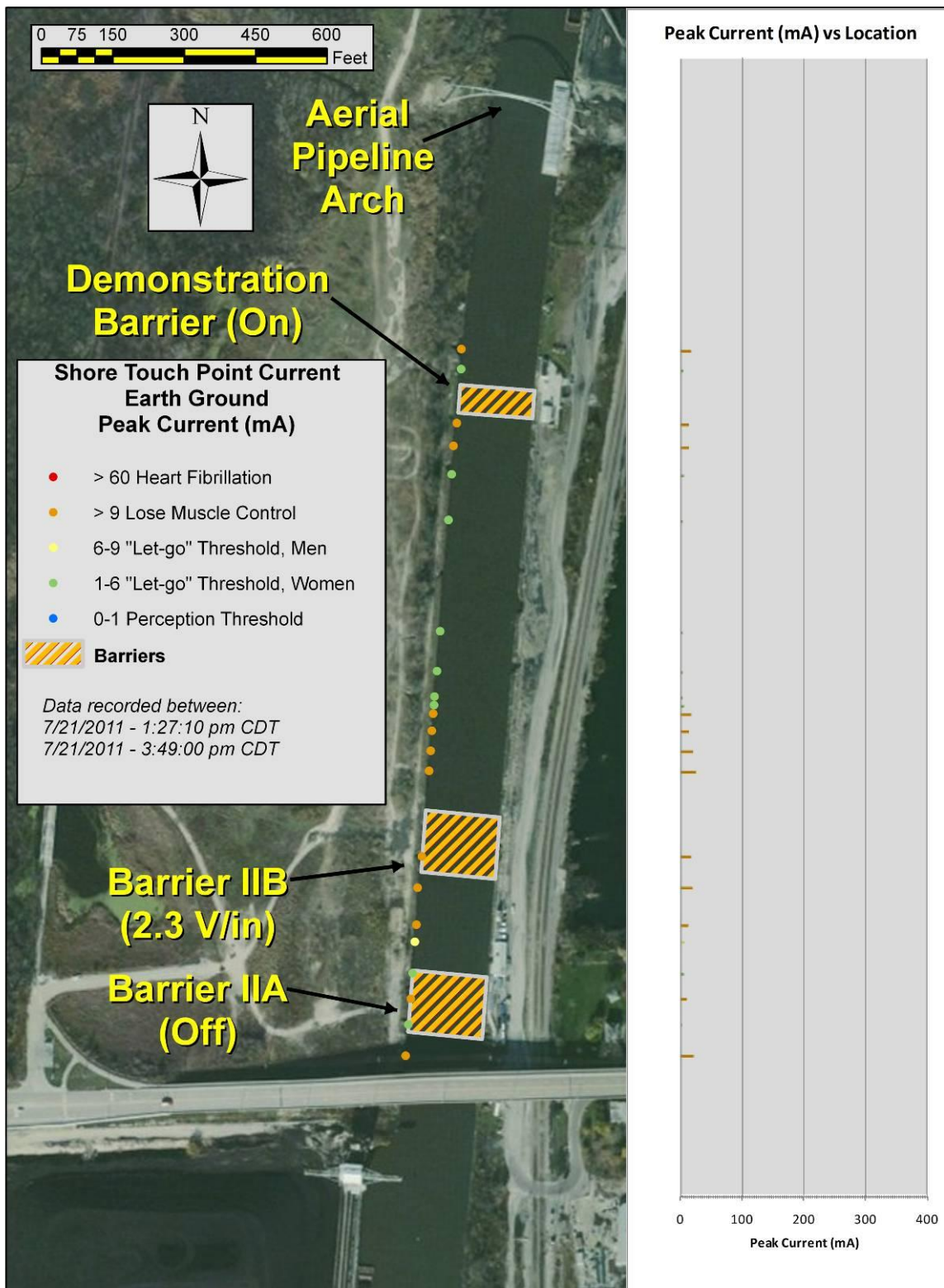
Figure 24. Results for shore touch-point current, “earth ground”, Barrier IIA “off”.
