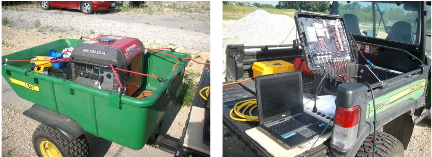
Figure 5. Shore touch-point data acquisition equipment set-up.
