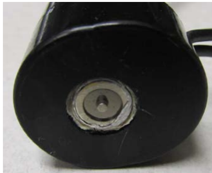
FIGURE 3. Image of the assembled probe. The black external housing is the coil and the microphone is secured in the middle of the coil. The magnet shown here is a cylindrical magnet.
