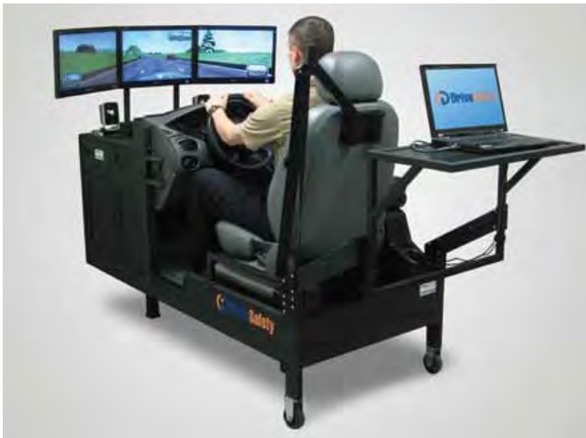
FIGURE 8-1. Adaptive driving simulator. Copyright 2010 DriveSafety, Inc. All rights reserved.
