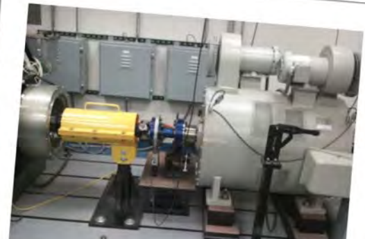
Commissioned a new four-quadrant dynamometer for characterization and testing of electric machines, e.g. hybrid electric propulsion motors
