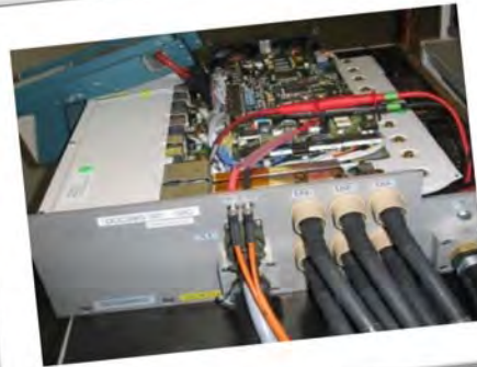
Bench tested Silicon Carbide (SiC) 150 kW DC-DC Battery-to-Bus (BTB) Converter
