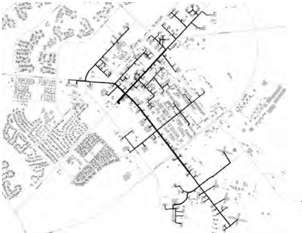
Figure 39. Design of the district heating network.
