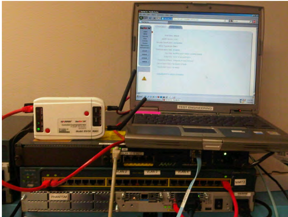
Figure 4. SecNet54 Radio Module Providing Tunneling Services to Switch. 1
