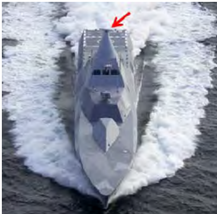
Figure 15. Pilot Radar on Visby-class Corvette (Radar Antenna--Red Arrow)
