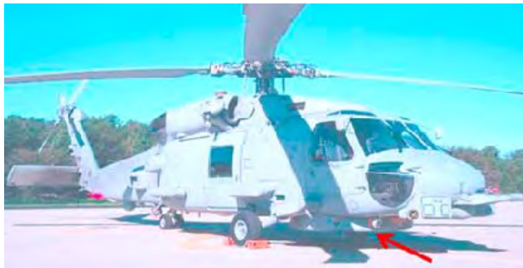
Figure 11. AN/APS-147 Radar (Antenna Under Helicopter Cockpit--Red Arrow)
