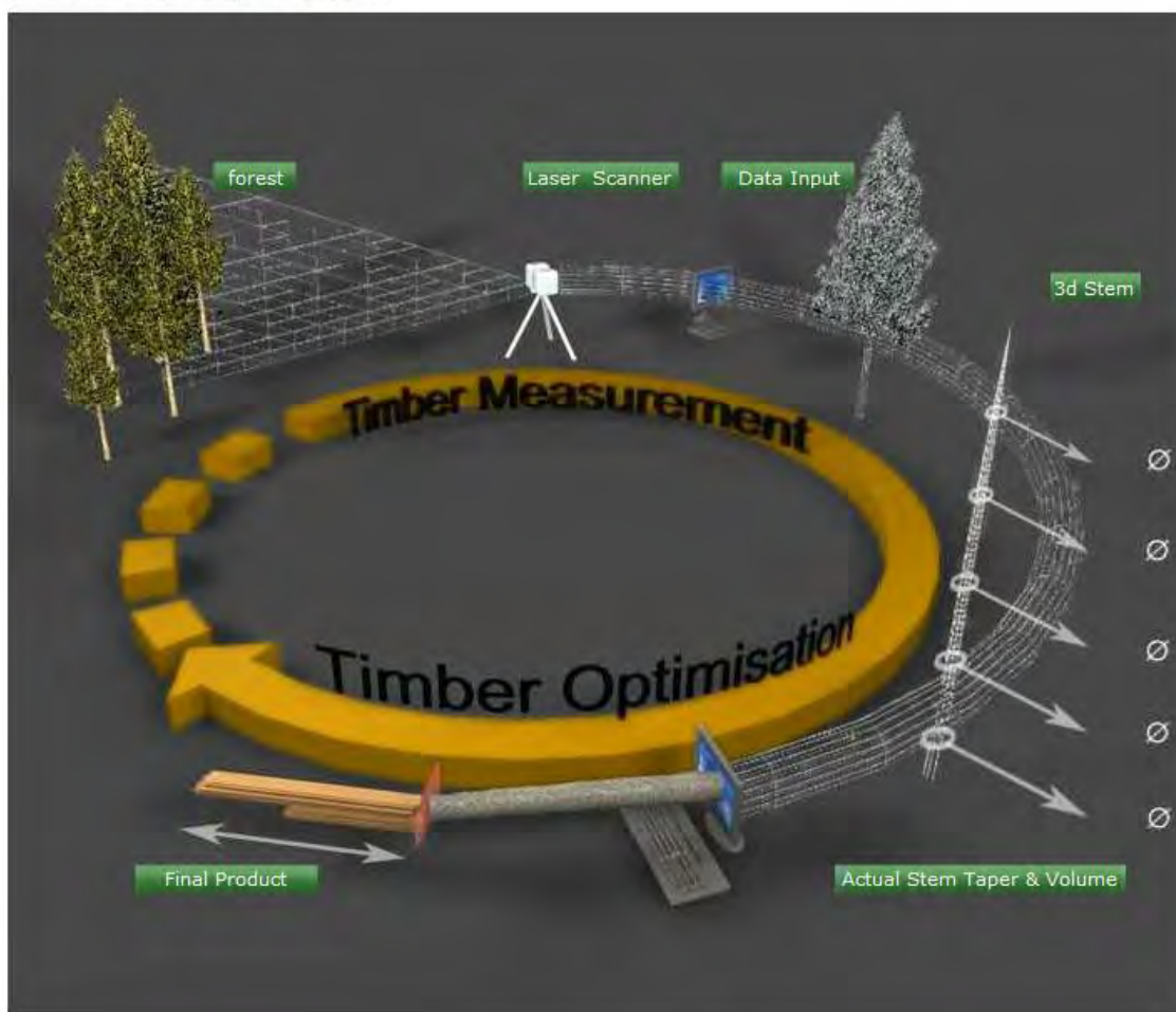
Figure 8. Description of specific method advocated by TreeMetrics software company for utilizing terrestrial LiDAR in timber measurement and optimization (From TreeMetrics, Ltd., 2011).
