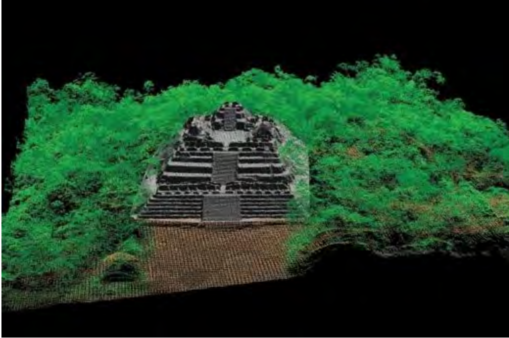
Figure 15. Rendering from airborne LiDAR point cloud surrounding Mayan pyramid (From Diaz, 2011)
