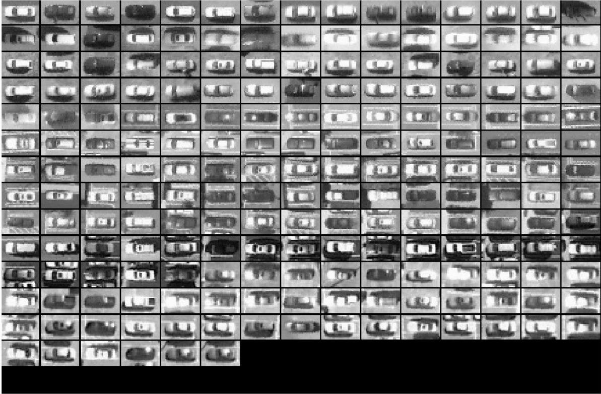
Figure 4.2: This shows the training set as it is provided to the OpenCV haar cascade training algorithm for the non-rotated cascade.
