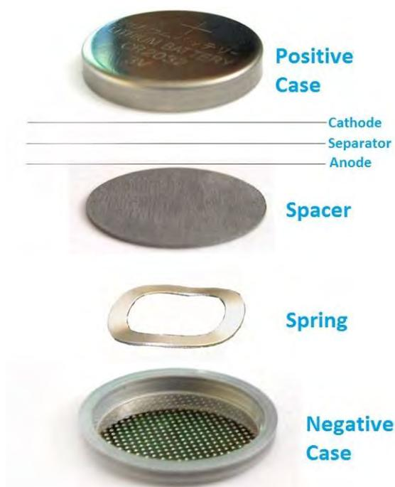
Figure 18. Button-type coin cell assembly schematic.
