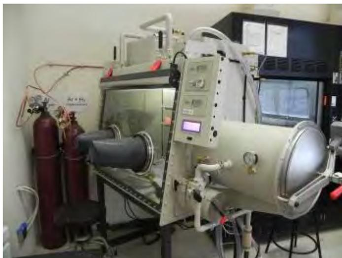
Figure 17. An Argon-filled glove box was used to prepare and assemble the coin cell batteries. The glove box prevents the electrodes from getting in contact with oxygen and moisture, both of which are known to reduce the cycle-life of Li-ion batteries.
