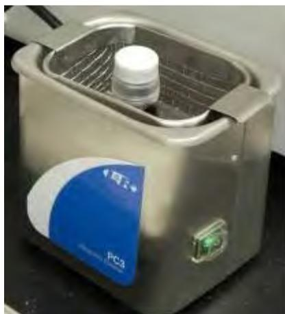
Figure 12. Sample vial containing a  $\text{LiFePO}_4$  slurry inside the ultrasonic bath. Each vial was sonicated for 30 minutes.
