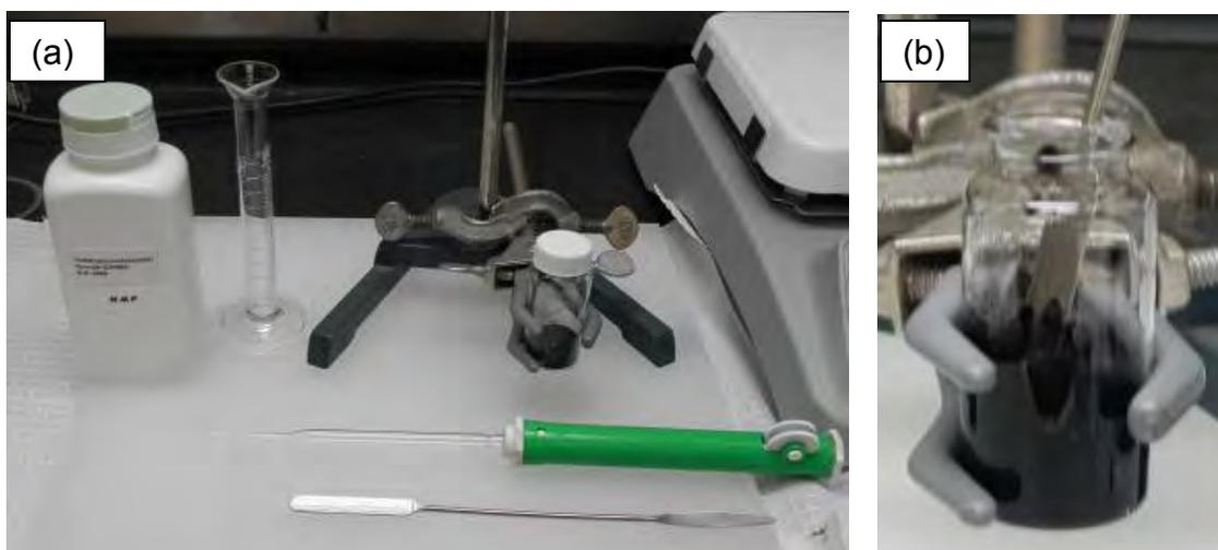
Figure 11. a) Slurry preparation setup under the fume hood with NMP solvent, glass pipette with dispenser, and the ball milled powder mixture containing  $\text{LiFePO}_4$ , acetylene black, and PVDF binder; and b) Prepared slurry after adding NMP solvent to the powder mixture.
