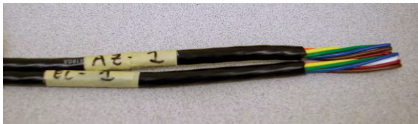
Figure 64. G-5500 AZ/EL Cable – Initial Strip
