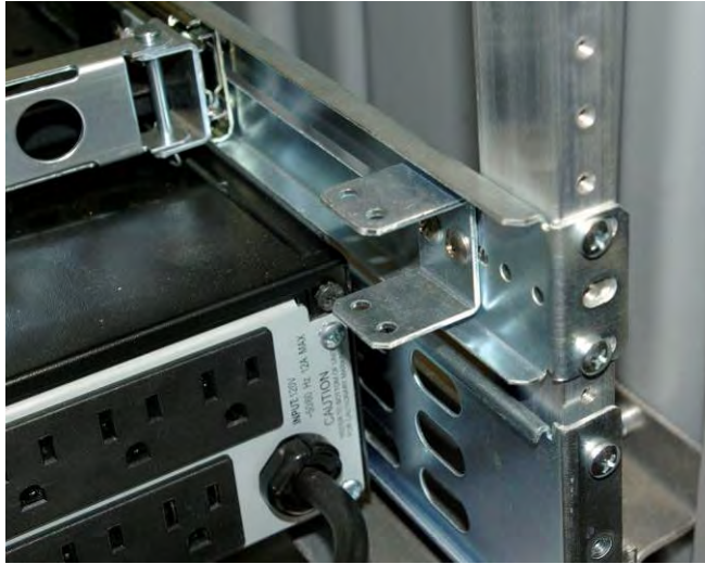
Figure 42. Sliding Rack Shelf–Rear Installation and U-Clip. This shelf is at position 19 and the U-Clip is on the same side as the UPS power cord.
