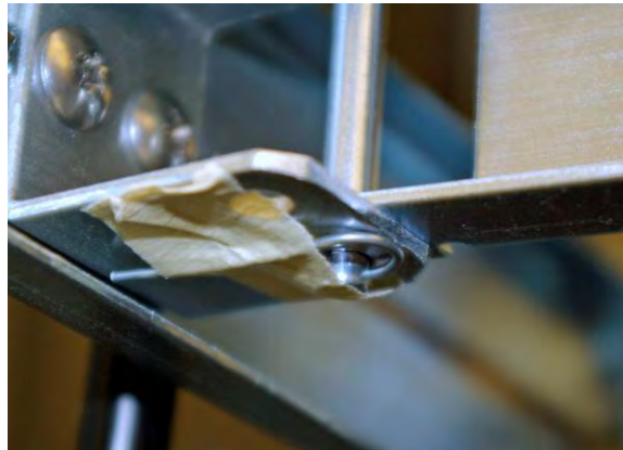
Figure 16. Double Captured, Taped Cotter Pin
