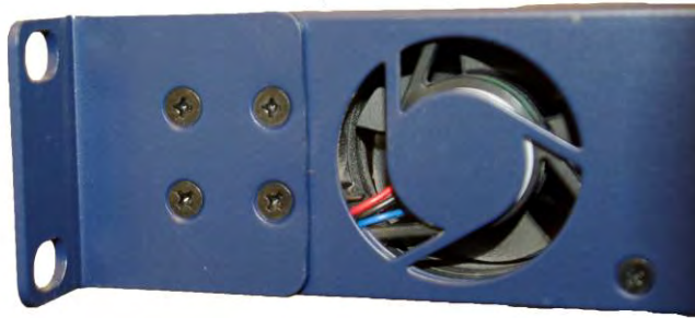
Figure 49. Network Switch – Rack Adapter
