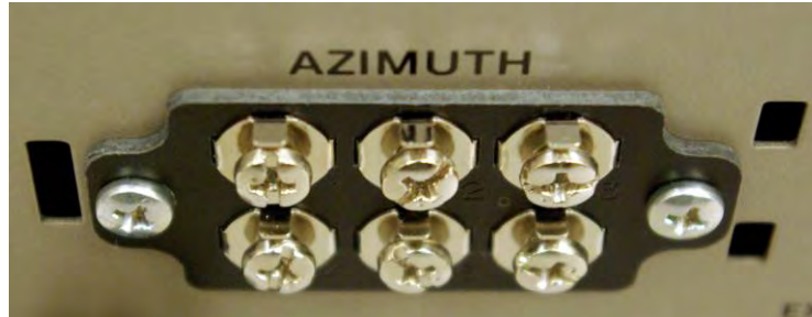
Figure 68. G-5500 – Screws Loosened but not Removed
