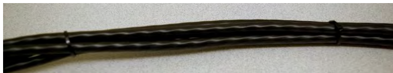
Figure 87. AZ/EL Cable – Zip Tie Spacing and No Twists
