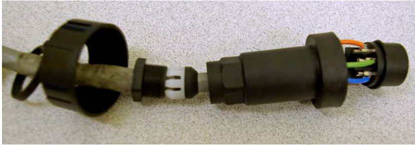
Figure 107. AZ/EL Cable – Wires Attached
