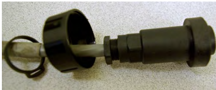
Figure 108. AZ/EL Cable – Connector Secured from Front and Rear
