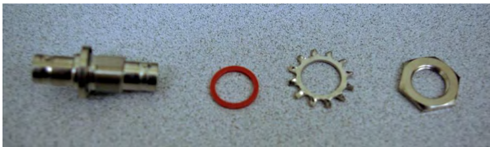
Figure 96. GPS Connector - Disassembled
