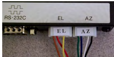
Figure 74. GS-232B – AZ/EL Connections
