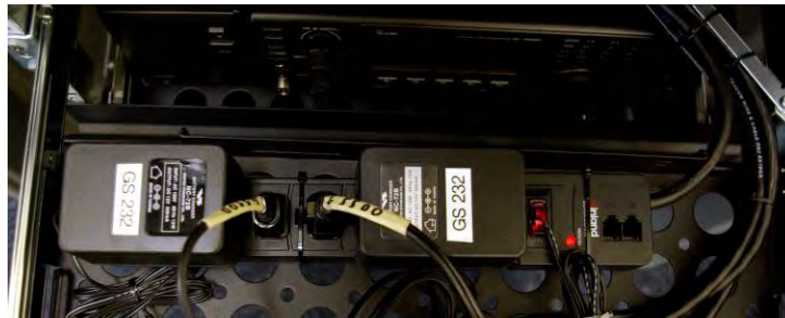
Figure 73. GS-232B and G-5500 – Power Connections
