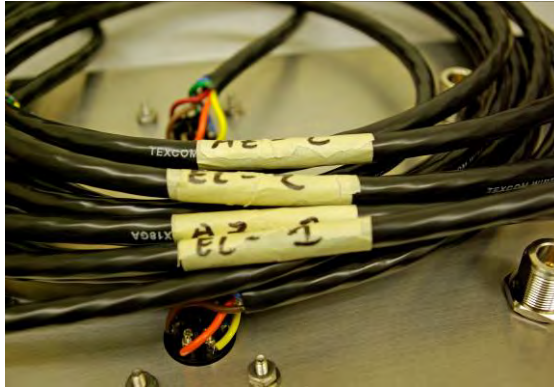
Figure 84. AZ/EL Cables – Wire Identifiers
