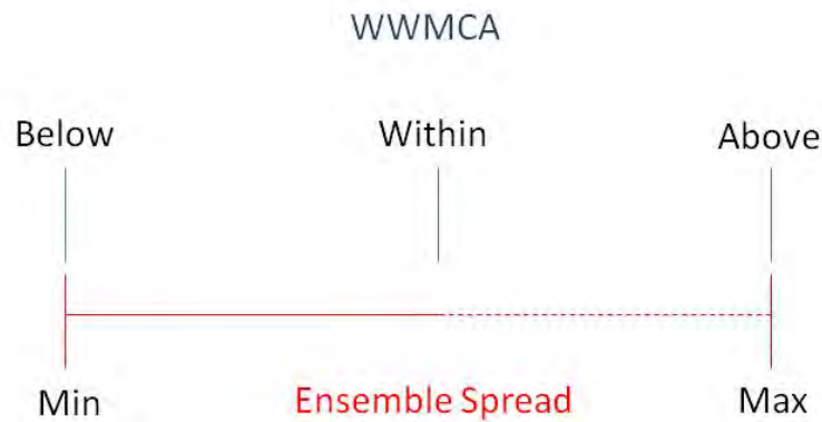
Figure 53. WWMCA Modification of Ensemble Spread. The ensemble spread (red line) is modified when the WWMCA cloud fraction fall below the value of the maximum ensemble-member analyses (Max).
