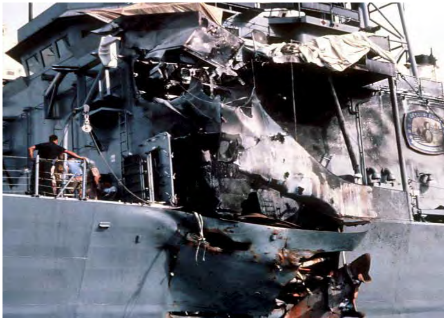
Figure 11. A View of the External Damage to the Stark's Port Side (From Navy Command, 1987 )
