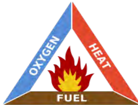
Figure 2. Requirements for Combustion (From Gustavb, 2006)
