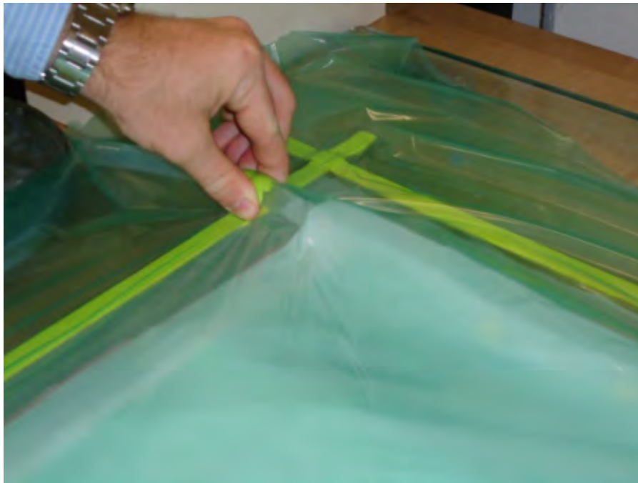
Figure 8. Composite Fabrication: Tucking the vacuum bag around suction hose interface.
