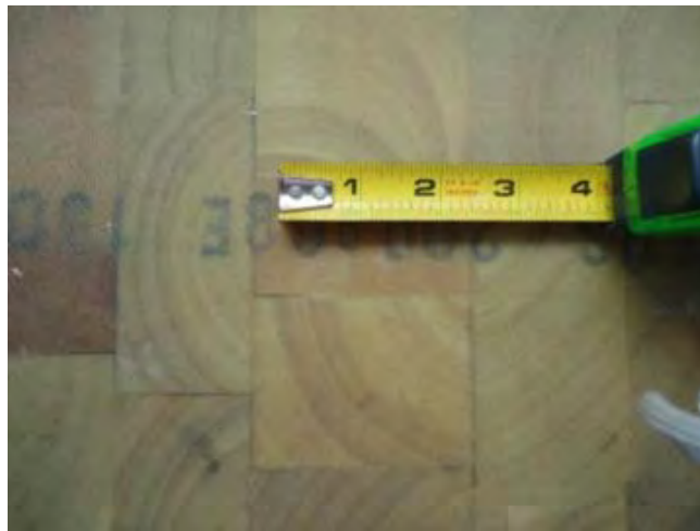
Figure 21. Sample Wet1 initial damage at 6 in drop height.
