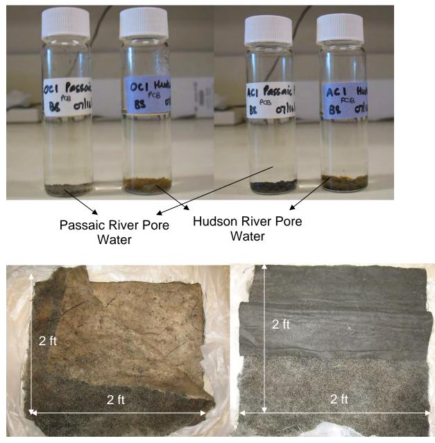
Reactive core mats drying at room temperature prior to sorbent separation
