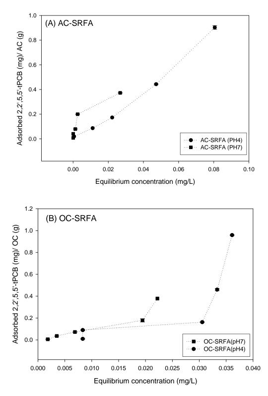
Adsorption of 2, 2', 5, 5'-tPCB in presence of Suwannee River FA at pH 4 and 7 (A) Activated carbon (B) Organoclay
