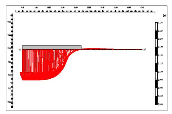
Figure 5.3-23. Horizontal profile of maximum sediment displacement under the uncoupled consolidation model.
