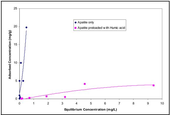
Figure 7.1-17. Adsorption isotherm for lead onto apatite.
