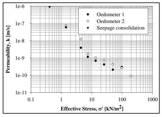
Figure 5.3-19. Permeability versus effective stress for Cottonwood Bay sediment.
