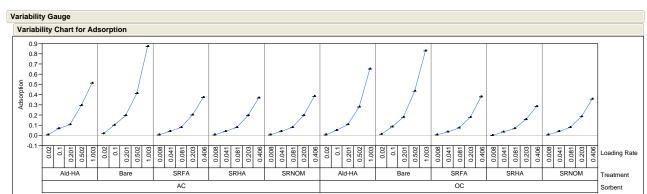
Model 1 detail: for 2, 2', 5, 5'-tPCB adsorption in presence of Ald-HA/ SRHA/ SRFA/ SRNOM
