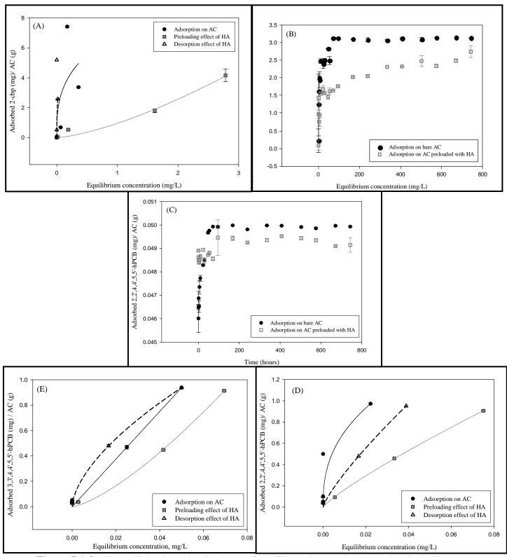
**Figure 7.1-2**. Freundlich adsorption isotherms for PCBs on bare activated carbon including preloading and desorption effects of humic acid: (A) 2-cbp, (B) 2,2',5,5'-tPCB (C) 3,3',4,4'-tPCB (D) 2,2',4,4',5,5'-hPCB and (E) 3,3',4,4',5,5'-hPCB.
