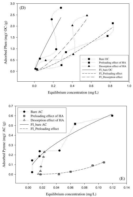
Figure 4.2 D-E: Freundlich Isotherms and actual trend of curves for adsorption on bare sorbents and preloading and desorption effect of humic acid: (d) Phenanthrene adsorption on organoclay (e) Pyrene adsorption on activated carbon
