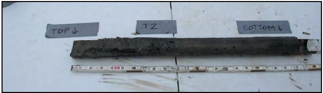
Figure I-3. Sediment core collected from treatment area T2 (mat with sand cap).
