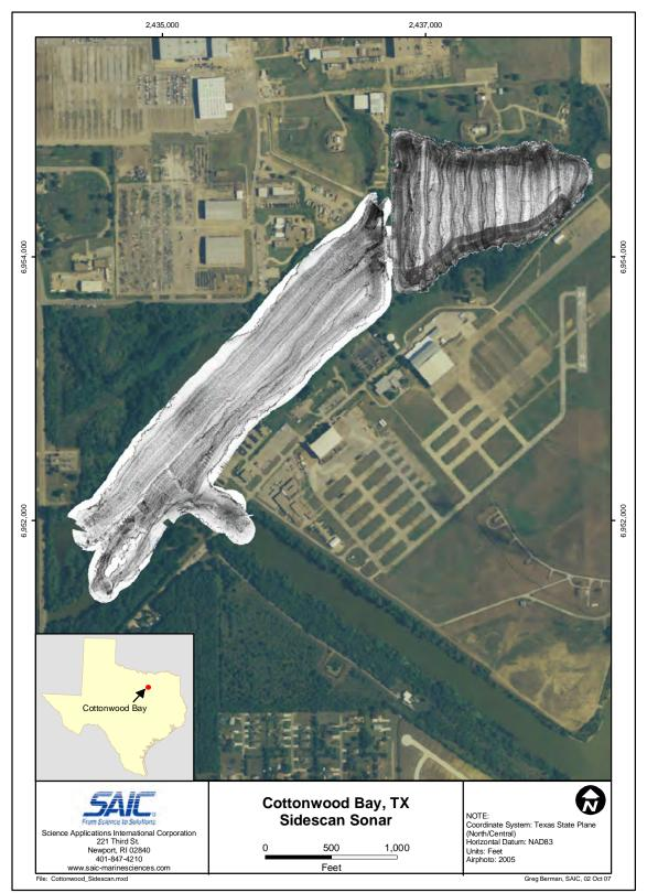
Figure 7.2-8. Complete side-scan sonar results for Cottonwood Bay.
