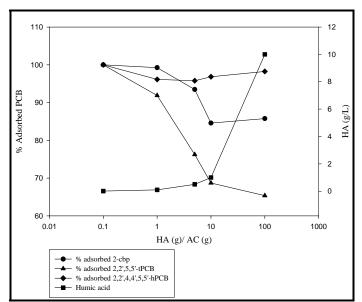
**Figure 7.1-5**. Effect of different loadings of humic acid on 2-chlorobiphenyl, 2,2',5,5'-tPCB and 2,2',4,4',5,5'-hPCB.
