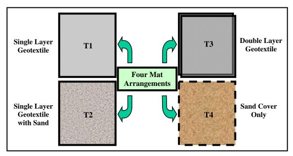
Figure 4.4-2. Various arrangements for prototype mat system testing.
