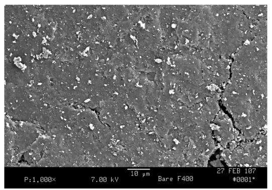
Coal based activated carbon: 1000 x magnifications
