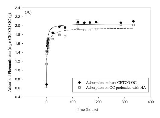
Figure 4.1A: Kinetics: Phenanthrene adsorption on organoclay
