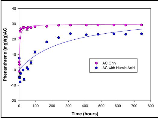
Figure 7.1-4. Kinetics of phenanthrene adsorption on activated carbon.
