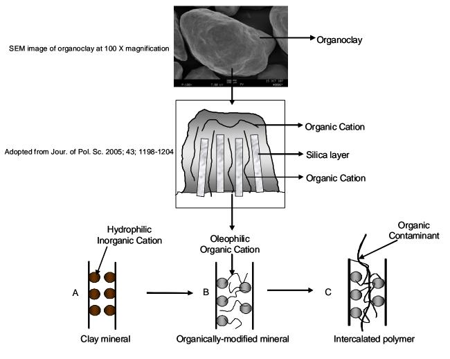
Mechanism of sorption onto organoclay
