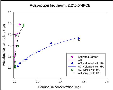
Figure 7.1-9. Adsorption isotherm of 2,2',5,5'-tetrachlorobiphenyl onto activated carbon.
