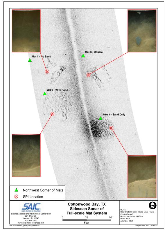
**Figure D-4**. Side-scan sonar mosaic of the prototype mat system with representative sediment profile images of each treatment area.
