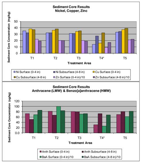
\*For area T4, the 0-4 in horizon represents predominantly the sand cap material and the 4-8 in horizon represents the natural sediment comparable to the surface horizon in other areas.
