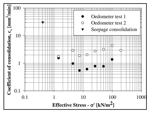
Figure 5.3-15. Coefficient of consolidation of Cottonwood Bay sediment.
