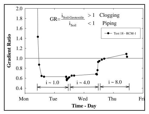
Figure 5.3-6. Gradient ratio test results for weathered geotextile mat RCM-1 after six months of soak time in Cottonwood Bay.
