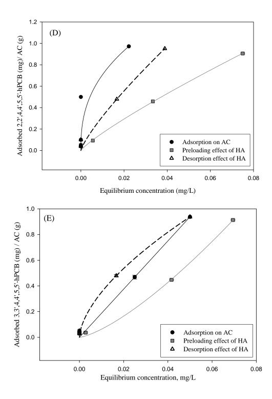
Figure 2.4 D - E. Freundlich Adsorption Isotherms for selected PCB congeners with bare AC and preloading and desorption effect of HA: (D) 2,2',4,4',5,5'-hPCB (E) 3,3',4,4',5,5'-hPCB
