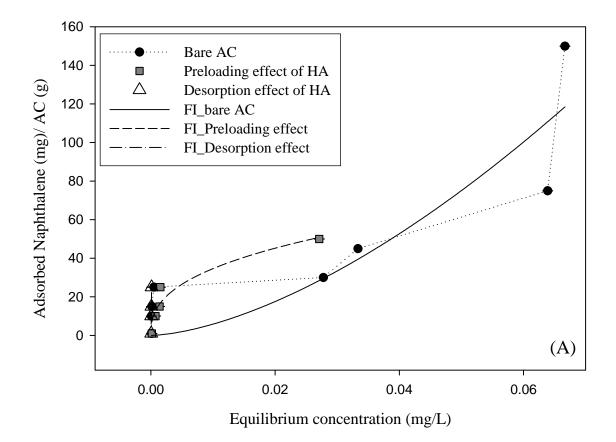
Figure 4.2 A: Freundlich Isotherms and actual trend of curves for adsorption on bare sorbents and preloading and desorption effect of humic acid: Naphthalene adsorption on activated carbon
