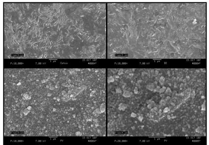
**Figure 6.1-2.** Scanning electron micrograph cross-section profiles of three different organoclays: CETCO (10K x magnification - top left), Biomin, Inc. (10K x magnification - top right) and Polymer Ventures (10K x magnification – bottom left and 20K x magnification - bottom right).
