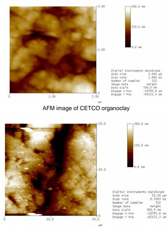
Atomic Force Micrographs produced to demonstrate the topography of organoclays
