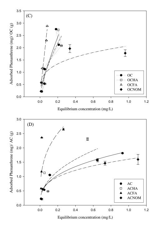
Adsorption of contaminants in presence of different fractions of natural organic matter (A) 2,2',5,5'-tPCB adsorption on OC (B) 2,2',5,5'-tPCB adsorption on AC (C) Phenanthrene adsorption on OC (D) Phenanthrene adsorption on AC (OC = Organoclay; AC = Activated Carbon; HA = Aldrich Humic Acid (pH 7.21); FA = Fulvic Acid (pH 4.02) and NOM = Natural Organic Matter (pH 4.12)
