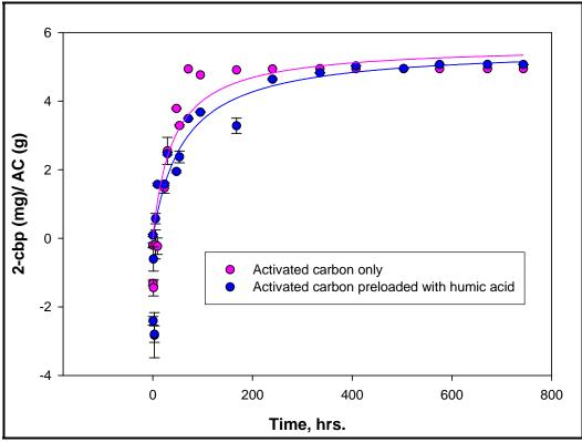
Figure 7.1-1. Kinetics of 2-chlorobiphenyl adsorption on activated carbon.
