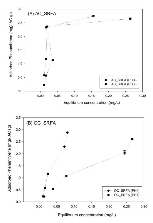
Adsorption of phenanthrene in presence of Suwannee River FA at pH 4 and 7 (A) Activated carbon (B) Organoclay
