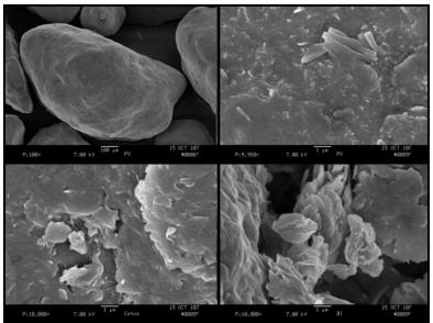
**Figure 6.1-1.** Scanning electron micrograph surface profiles of three different organoclays: Polymer Ventures (100x magnification - top left and 10K x magnification - top right), CETCO (10K x magnification - bottom left) and Biomin, Inc. (10K x magnification - bottom right).
