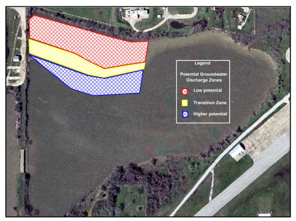
Figure 5.2-5. Potential groundwater discharge zones for Cottonwood Bay.
