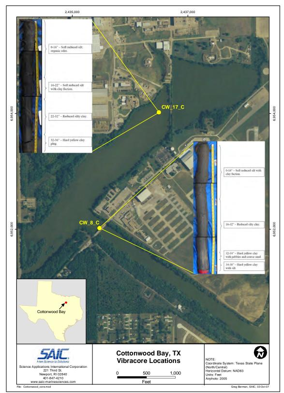
**Figure 7.2-14**. Locations and field photographs of the sediment vibracores collected from Cottonwood Bay West (Station CW-8 and Station CW-17).
