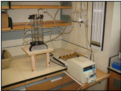
Figure 6.3-4. Geotextile permeability column experimental setup.
