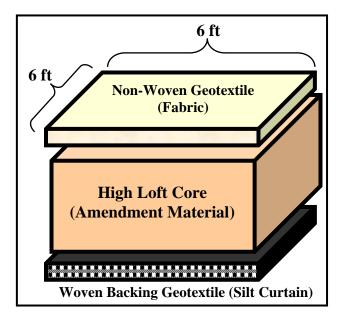
Figure 4.3-1. Construction diagram of small-scale geotextile test mats.
