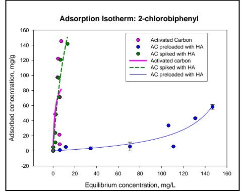
Figure 7.1-8. Adsorption isotherm of 2-chlorobiphenyl onto activated carbon.
