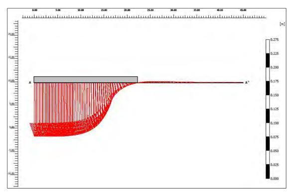
Figure 5.3-28. Horizontal profile of the maximum sediment displacement under the coupled model.
