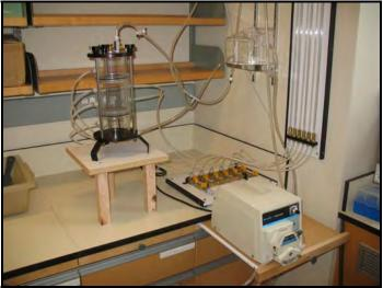
Figure 6.3-1. Permeability column test setup.
