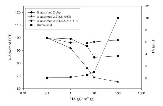
Figure 2.8: Effect of different loadings of HA on adsorption of 2-chlorobiphenyl; 2, 2', 5, 5'-tPCB and 2, 2', 4, 4', 5, 5'-hPCB
