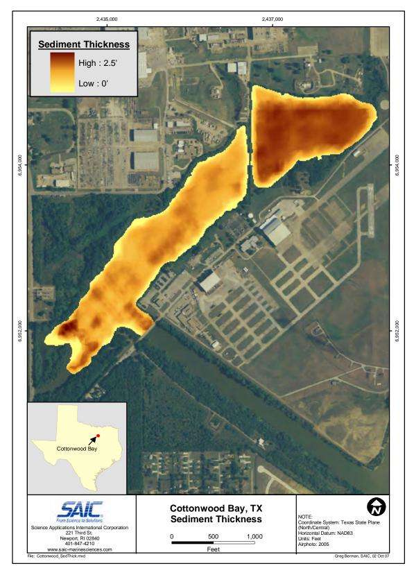
**Figure 7.2-6**. Sediment thickness results for Cottonwood Bay developed from sub-bottom profile data.
