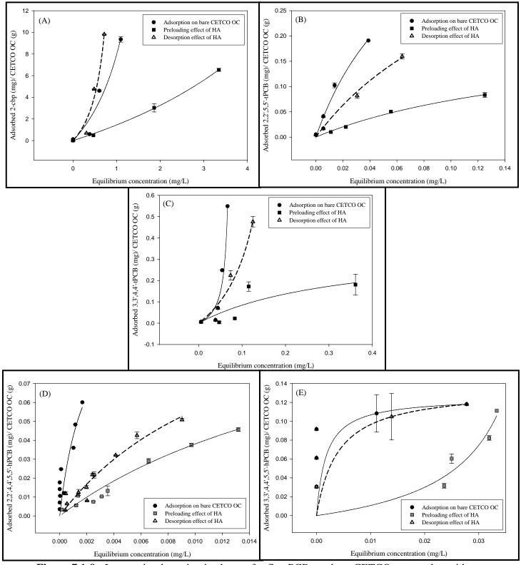
**Figure 7.1-9**. Langmuir adsorption isotherms for five PCBs on bare CETCO organoclay with preloading and desorption effects of humic acid: (A) 2-cbp, (B) 2,2',5,5'-tPCB, (C) 3,3',4,4'-tPCB, (D) 2,2',4,4',5,5'-hPCB and (E) 3,3',4,4',5,5'-hPCB.
