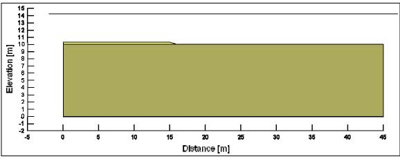
Figure 6.3-8. Geometry of a typical reactive mat application for finite element modeling.
