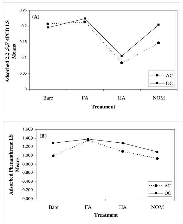
Statistical analysis of performance of sorbents (A) 2, 2', 5, 5'-tPCB adsorption on AC and OC in presence of HA/ FA/ NOM (B) Phenanthrene adsorption on AC and OC in presence of HA/ FA/ NOM (AC = activated carbon; OC = organoclay)
