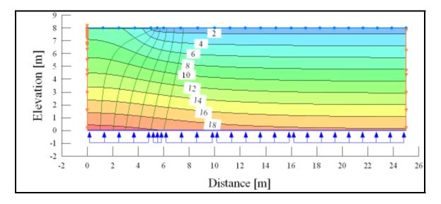
**Figure C-10**. Pressure head contours (m) and flow paths ( $k_{GT} = 0.0001 \text{ x } k_{SED}$ )
