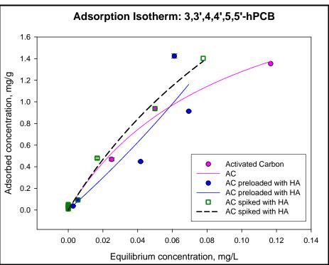
**Figure 7.1-13.** Adsorption isotherm of non-coplanar 2,2',4,4',5,5'–hexachlorobiphenyl onto activated carbon.
