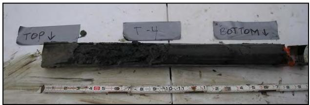
Figure I-5. Sediment core collected at treatment area T4 (sand cap only).
