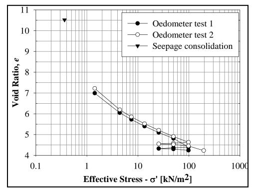
Figure 5.3-14. Consolidation of Cottonwood Bay sediment; void ratio versus effective stress.
