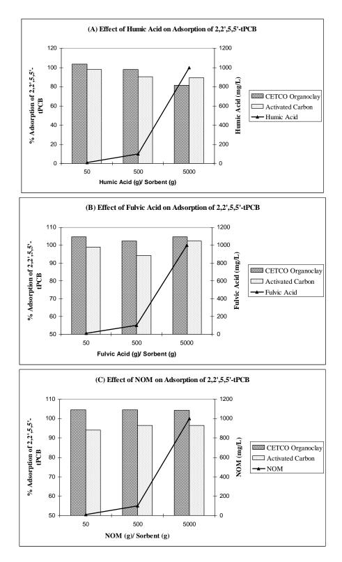
Figure 5.7A-C: Comparison of performance of organoclay and activated carbon for adsorption of 2, 2', 5, 5'-tPCB in the presence of humic acid, fulvic acid and natural organic matter normalized to adsorption on bare materials.
