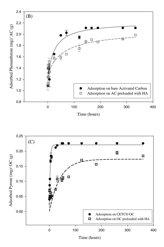
Figure 4.1B-C: Kinetics of adsorption: (B) Phenanthrene adsorption on activated carbon (C) Pyrene adsorption on organoclay
