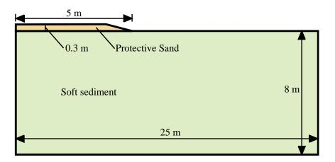
Figure C-1. Geometry of a generic reactive cap site for consolidation modeling (not to scale).
