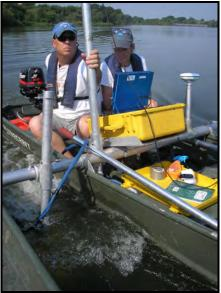
Figure 6.2-1. Bathymetry and sub-bottom transducer deployed from dual jon-boat survey craft.
