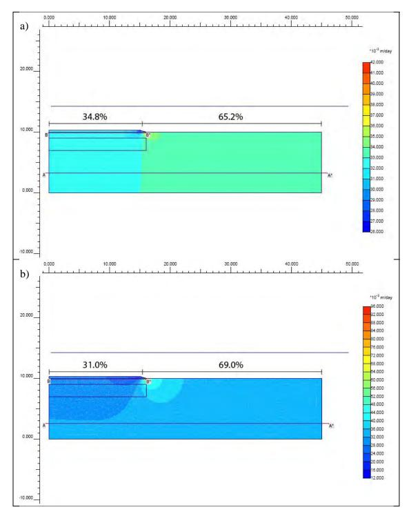
Figure 5.3-26. Specific discharge for an unclogged mat (a) and a clogged mat (b) under the uncoupled seepage model.
