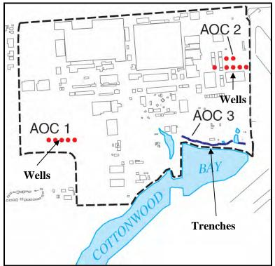
**Figure 7.2-4.** Locations of remedial wells and trenches at the Cottonwood Bay site (modified from Barker and Braun 2000).
