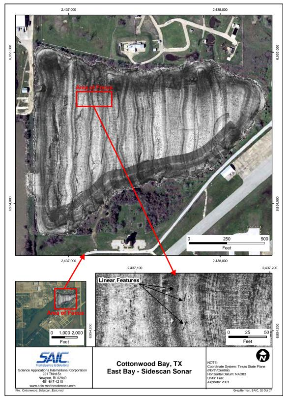
Figure 7.2-9. Side-scan sonar results for Cottonwood Bay East showing features of interest.
