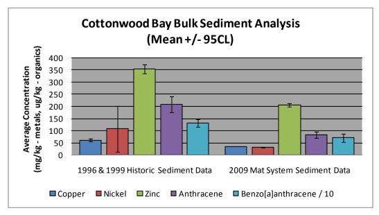
Figure 5.4-10. Historic and recent bulk sediment analytical results for select metals and organics at the prototype mat system area in Cottonwood Bay.
