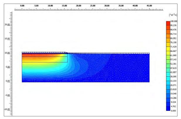
Figure 5.3-27. Sediment settlement due to mat deployment under the coupled model.
