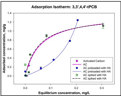
Figure 7.1-11. Adsorption isotherm for 3,3',4,4'-tetrachlorobiphenyl onto activated carbon.
