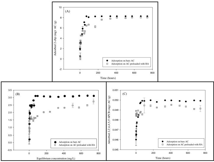
**Figure 7.1-1**. Kinetics of adsorption of different PCB congeners on coconut shell activated carbon in the presence and absence of humic acid: (A) 2-chlorobiphenyl, (B) 2,2',5,5'-tetrachlorobiphenyl and (C) 2,2',4,4',5,5'-hexachlorobiphenyl.
