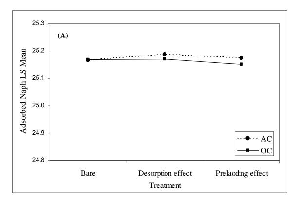
Figure 4.3 A: Least square means plot for comparison of performance of organoclay and activated carbon for adsorption of naphthalene
