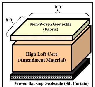
Figure 6.3-1. Construction diagram of small-scale geotextile test mats.
