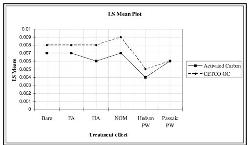
**Figure 7.1-16**. Least square mean plot to compare the effects of Passaic River sediment pore water, Hudson River sediment pore water, humic acid, fulvic acid and natural organic matter on the adsorption of 2,2',5,5'-tetrachlorobiphenyl by organoclay and activated carbon.
