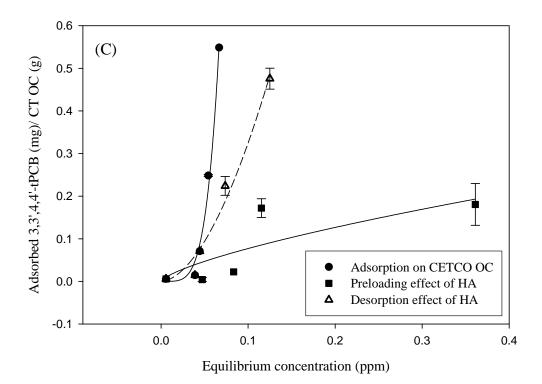
Figure 3.5C: Freundlich adsorption isotherms for adsorption of tetrachlorobiphenyl in presence and absence of humic acid: 3, 3', 4, 4'- tPCB adsorption on CETCO organoclay
