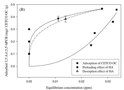
Figure 3.6B: Freundlich adsorption isotherms for adsorption of hexachlorobiphenyl on CETCO organoclay in presence and absence of humic acid: 3, 3', 4, 4', 5, 5'-hPCB
