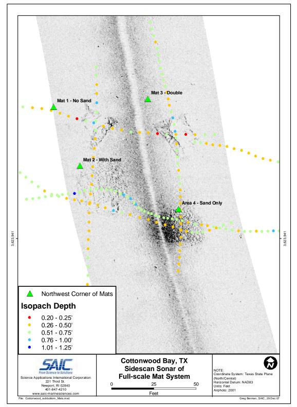
Figure D-3. Side-scan sonar mosaic of the prototype mat system with the sub-bottom isopach depth below the sediment-water interface of the uppermost sediment layer.
