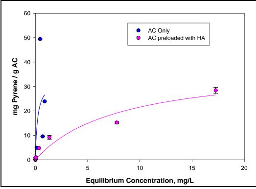
Figure 7.1-16. Adsorption isotherm for pyrene onto activated carbon.
