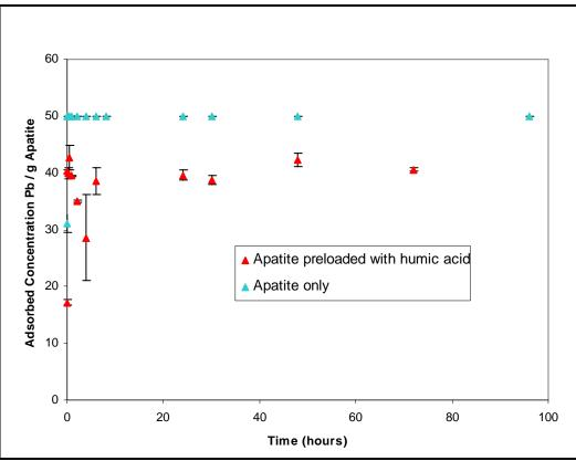
Figure 7.1-7. Kinetics of lead adsorption on apatite.
