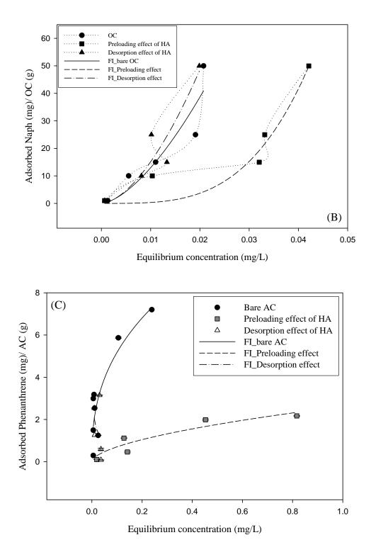
Figure 4.2 B-C: Freundlich Isotherms and actual trend of curves for adsorption on bare sorbents and preloading and desorption effect of humic acid: (b) Naphthalene adsorption on organoclay (c) Phenanthrene adsorption on activated carbon
