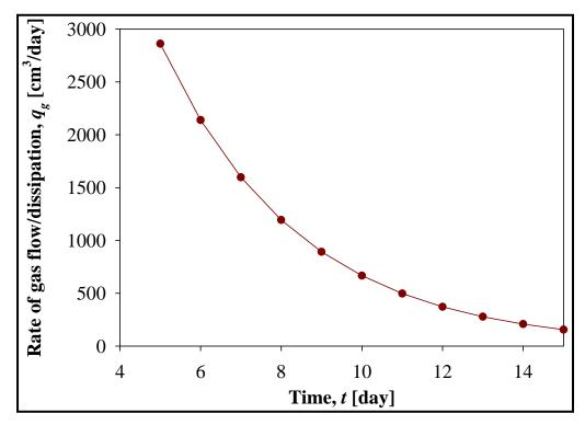
Figure 5.3-32. Flow/dissipation rate of gas versus time per square meter of geotextile.
