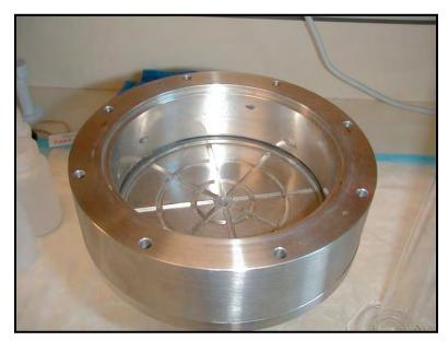
Figure 4.1-1. Experimental column for reactive mat flow-through testing.
