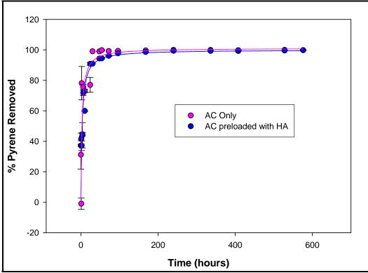
Figure 7.1-5. Kinetics of pyrene adsorption on activated carbon.
