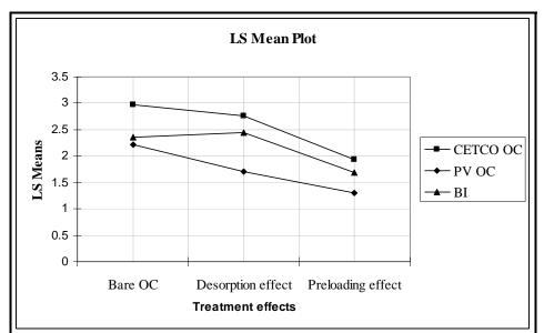
Figure 7.1-13. Least square mean plot to compare the effects of different humic acid treatments on the performance of three different organoclays in sequestering 2-chlorobiphenyl.
