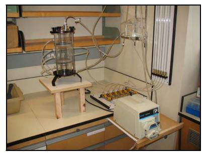
Figure 4.3-4. Geotextile sediment gradient ratio column experimental setup.
