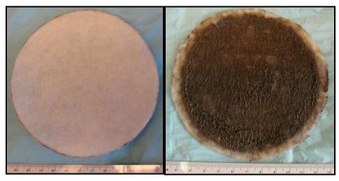
Figure 4.3-6. Comparative images of a geotextile sample before (left) and after (right) a gradient ratio test.
