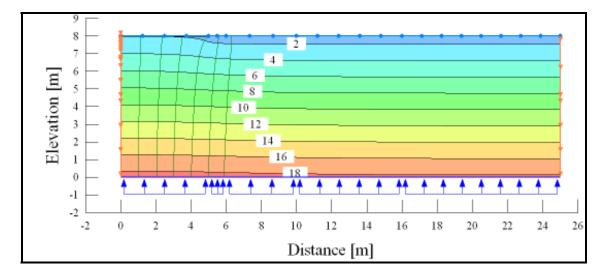
**Figure C-8**. Pressure head contours (m) and flow paths ( $k_{GT} = 0.01 \text{ x } k_{SED}$ ).
