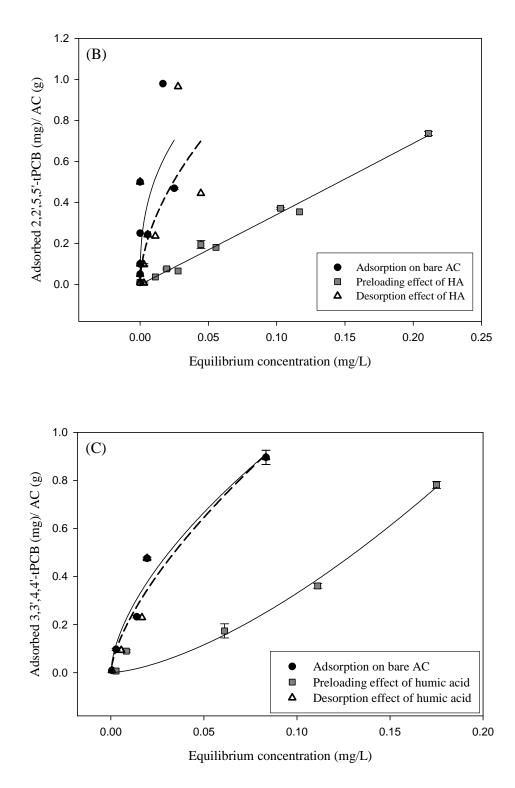
Figure 2.4 B - C. Freundlich Adsorption Isotherms for selected PCB congeners with bare AC and preloading and desorption effect of HA: (B) 2, 2', 5, 5'-tPCB (C) 3, 3', 4, 4'-tPCB
