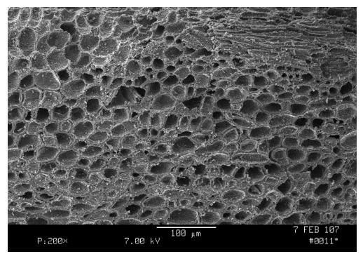
Coconut shell activated carbon: 200 x magnifications
