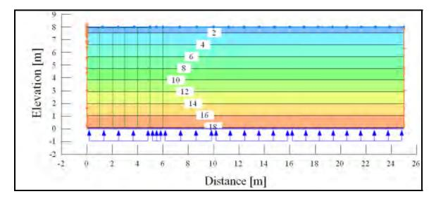
**Figure C-6**. Pressure head contours (m) and flow paths ( $k_{GT} = 1 \times k_{SED}$ ).
