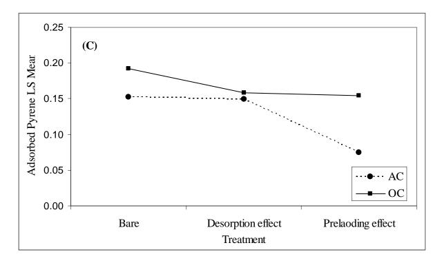
Figure 4.3 C: Least square means plot for comparison of performance of organoclay and activated carbon for adsorption: Pyrene
