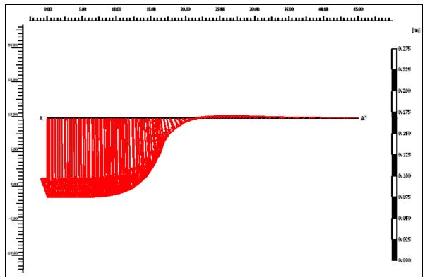
**Figure 7.3-8**. Horizontal profile of maximum sediment displacement under the uncoupled consolidation model.
