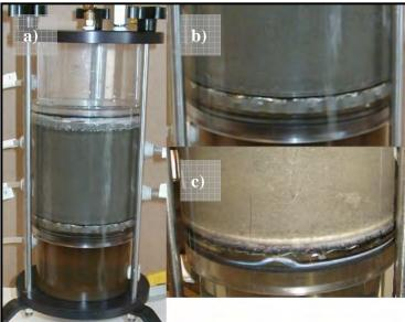
**Figure 6.3-5.** Detailed photograph of geotextile permeability test column showing (a) permeameter for gradient ratio tests, (b) geotextile-sediment contact and (c) mat-sediment contact.
