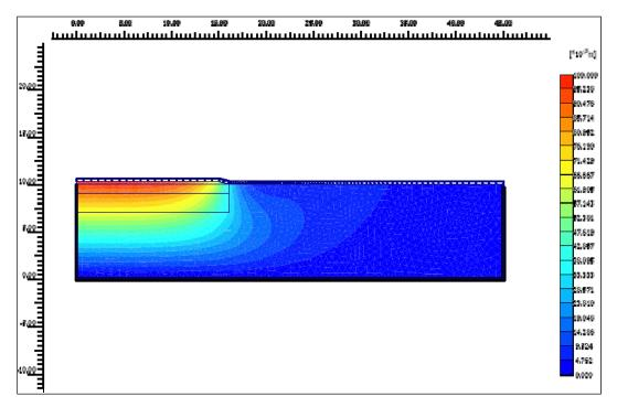
Figure 5.3-22. Settlement due to mat deployment after 95% sediment consolidation under the uncoupled model.
