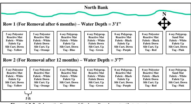
Figure 6.3-3. Schematic diagram of final small-scale geotextile test mat arrangement.
