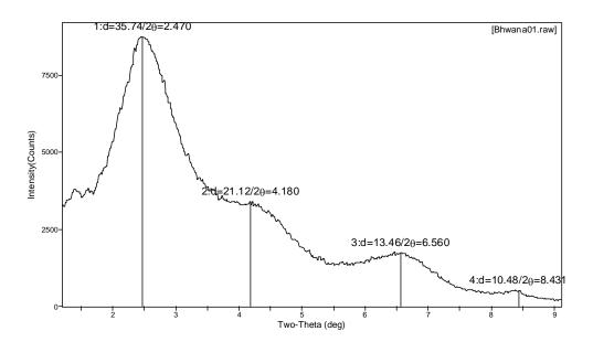
Figure 3.1.3: 2d SAXS scan for determination of d-spacing
