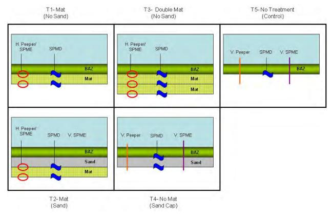
Figure 4.4-3. Vertical passive sampler layout in Cottonwood Bay.
