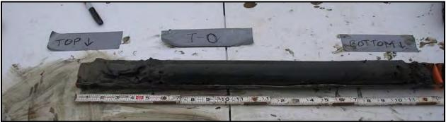
Figure I-7. Sediment core collected at area T0 (between all treatments).
