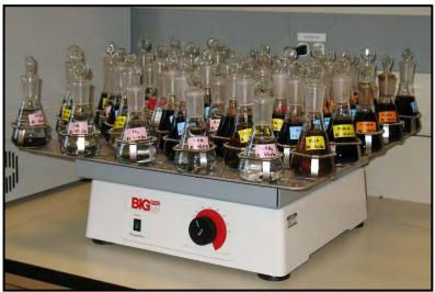
Figure 6.1-2. Batch experiments using activated carbon and organic contaminants.
