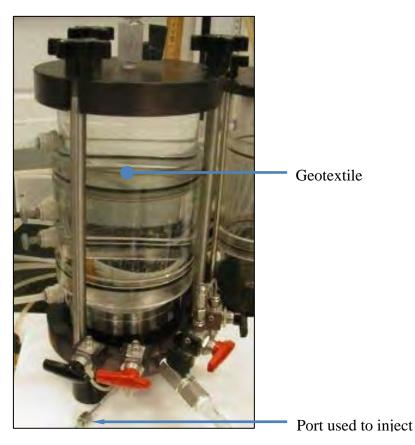
Figure 4.3-10. Permeameter setup for gas permeability testing.
