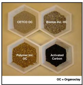
Figure 6.1-1. Reactive capping materials for organic contaminant sequestration.
