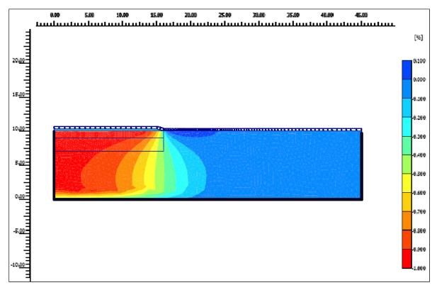
Figure 5.3-24. Volumetric strain after 95% consolidation under the uncoupled consolidation model.
