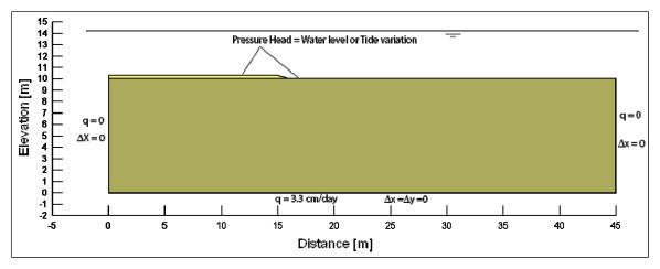
Figure 4.3-9. Summary of the boundary conditions for finite element modeling.
