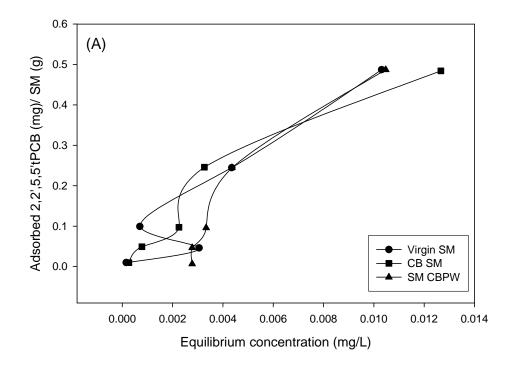
Figure 5.5 A: Comparison of bare sorbent mixture with the sorbent mixture obtained from reactive core mats deployed in Cottonwood Bay for 6 months: 2, 2', 5, 5'-tPCB adsorption(SM = Sorbent mixture; CB = Cottonwood Bay; and PW = Porewater)
