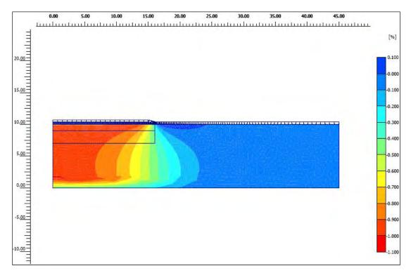
Figure 5.3-29. Volumetric strain under the coupled model.
