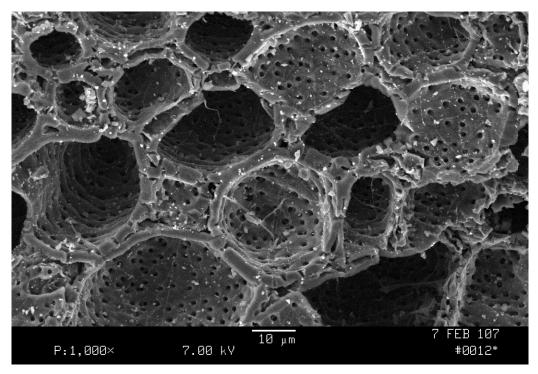
Coconut shell activated carbon: 1000 x magnifications
