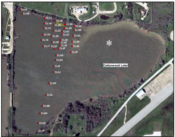
Figure 7.2-15. Trident probe stations for the Cottonwood Bay groundwater seepage survey.
