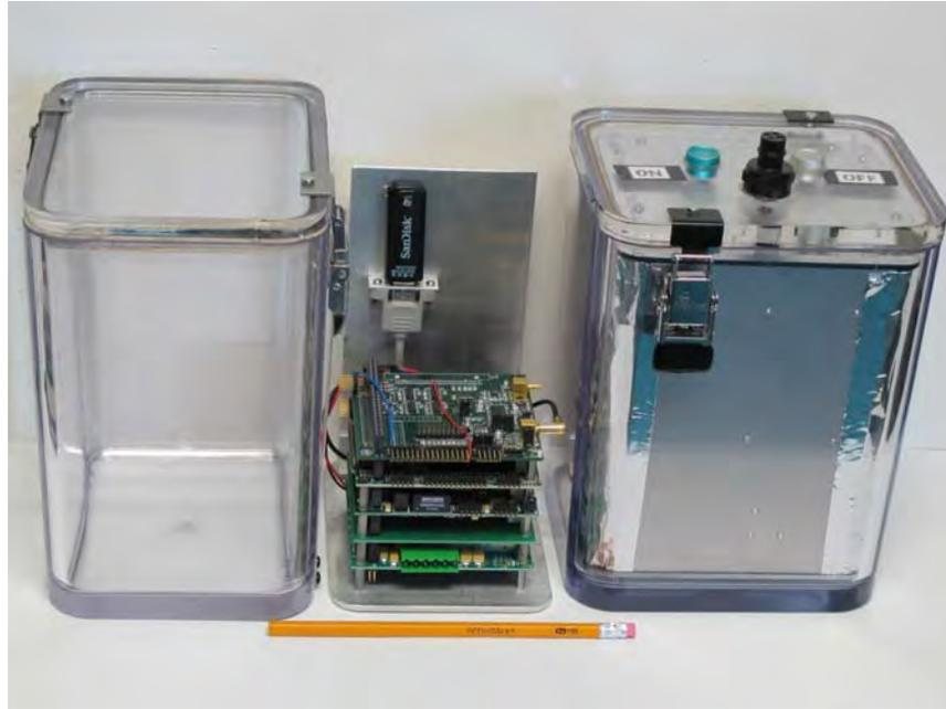
**Figure 14.** Laser-based Fluorescence Induction and Relaxation (FIRE) sensor for ROV/DSV platform. (Right) – Optical unit with a diode laser excitation source and large-aperture fluorescence collection optics; (Middle) – Electronic package with a computer board, control and data acquisition module, and power supply; (Left) – Housing for the electronic package.
