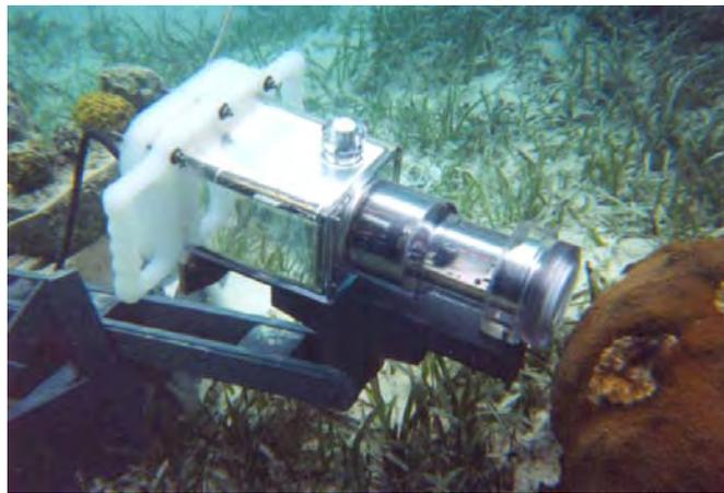
**Figure 3.** Diver-operated (top) and moored (bottom) FIRE Fluorometer Systems.
