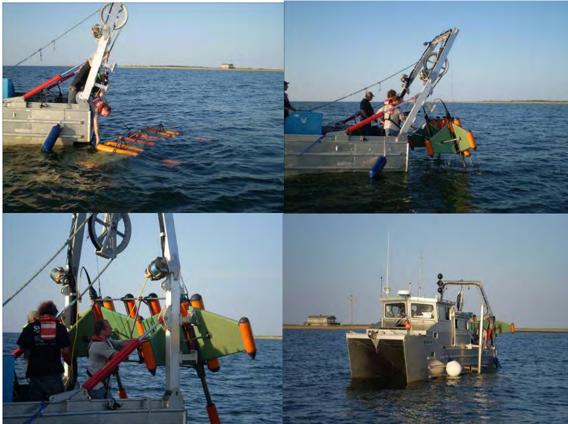
Figure 7-1. MGA Sequence of Recovery
