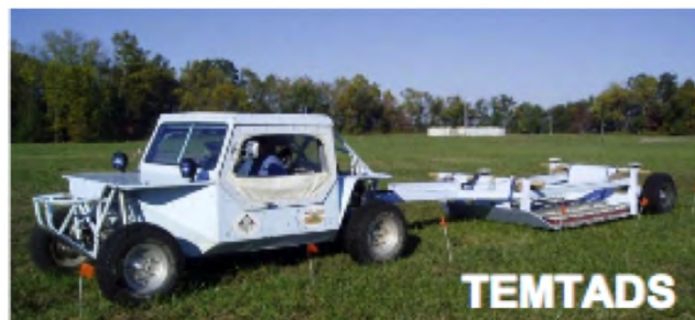
Figure 17: Nova Research Inc. operated the TEMTADS at the former Camp Butner. Taken from [51].
