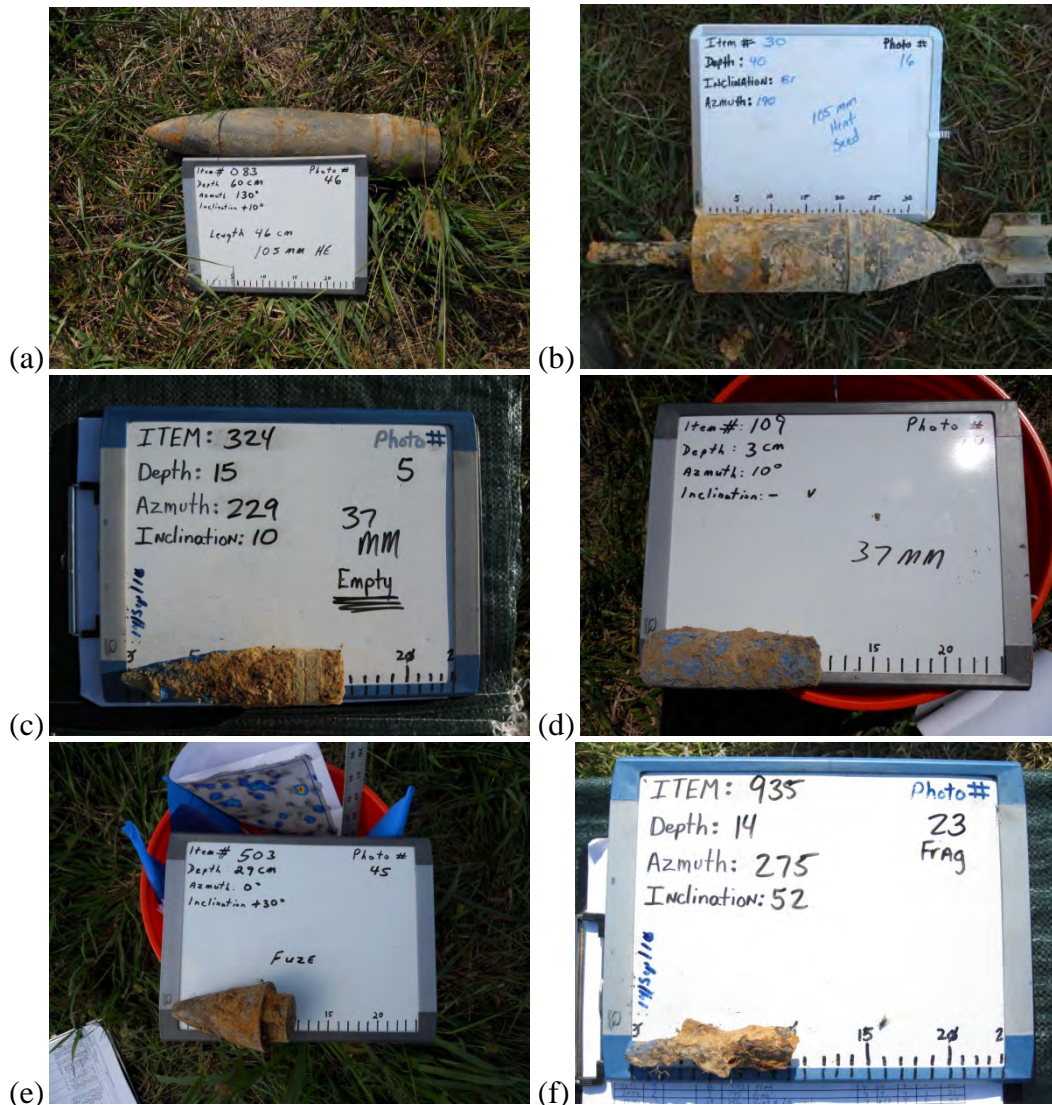
Figure 20: Photographs of recovered targets: (a) 105 mm projectile, (b) 105 mm HEAT projectile, (c) 37 mm projectile with driving band, (d) 37 mm projectile without driving band, (e) M48 fuze, and (f) scrap metal from a previously exploded munition. The targets in (a)–(e) were labeled “TOI”; the target in (f) was labeled “Non-TOI.”
