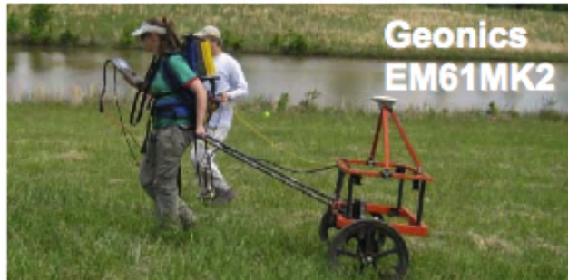
Figure 8: NAEVA Geophysics Inc. operated the EM61-Mk2 cart at the former Camp Butner. Taken from [51].
